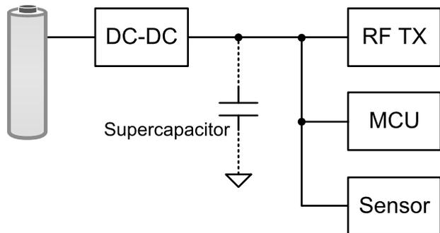
**Figure 1. Power Tree of a Battery-Powered Wireless Sensor**
