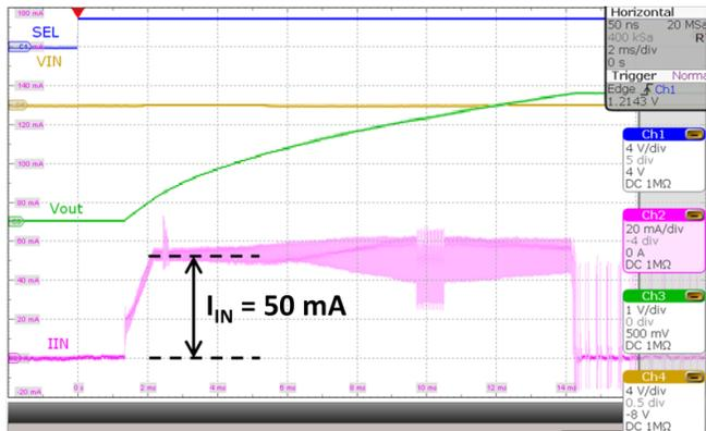
**Figure 3. Inrush Current Limited at 50 mA**
