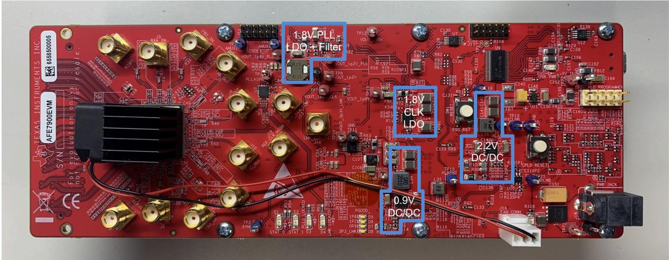
**Figure 1-3. Image of top of Original board with Switchers and LDO's outlined in Blue**
