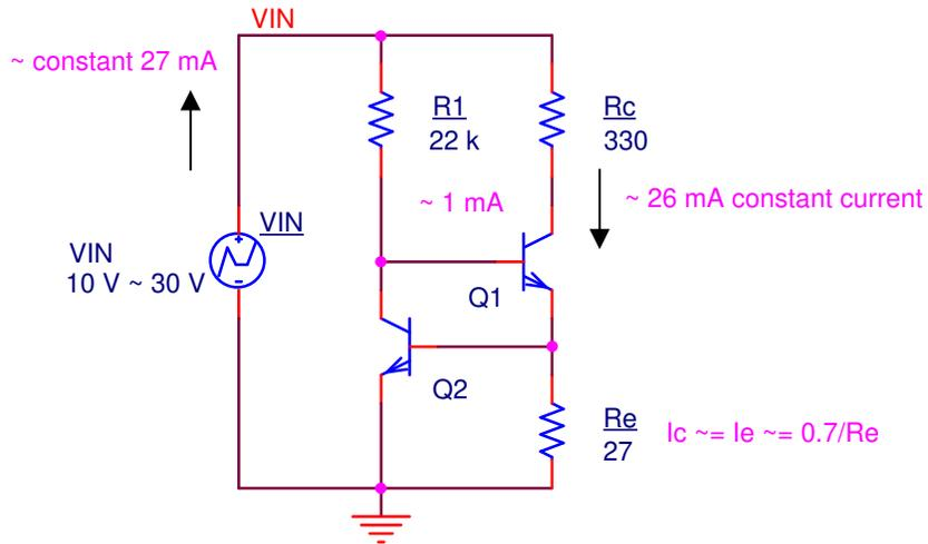
Figure 3-3. A Simple 27mA BJT Constant Current Source
