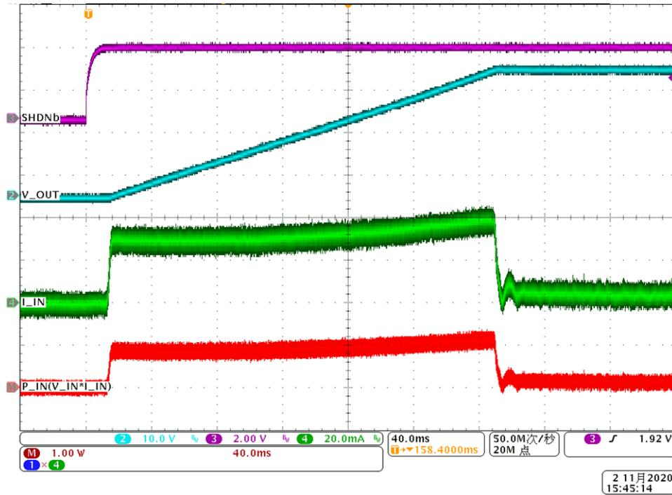
Figure 5-5. Start-up Inrush Current Control Waveforms at 30 V Input, 9Kohm Load
