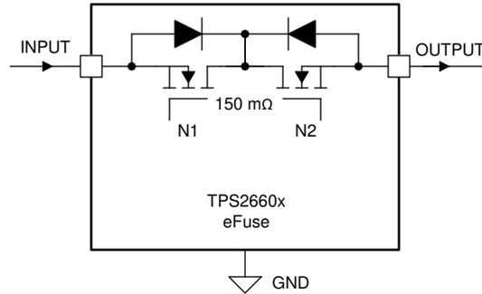
**Figure 2-3. TPS2660x - Back to Back FETs for Reverse Current Protection**
