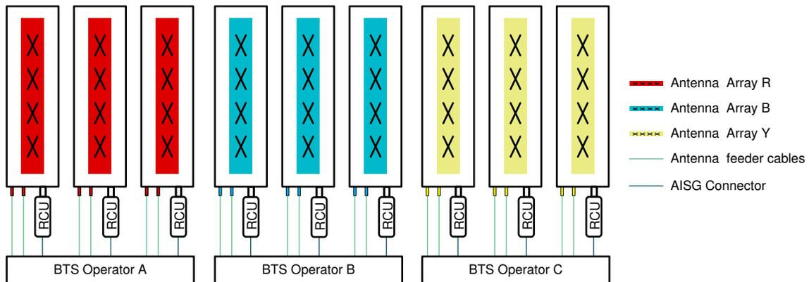
**Figure 1-1. Single-band Antenna Deployment for Single Mode of Three Operators**
