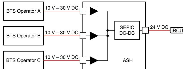
**Figure 2-1. ORing Diodes Solution for ASH PowerPath Management**
