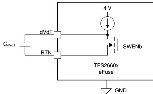
**Figure 2-4. Output Slew Rate Control Set by  $C_{dVdT}$**
