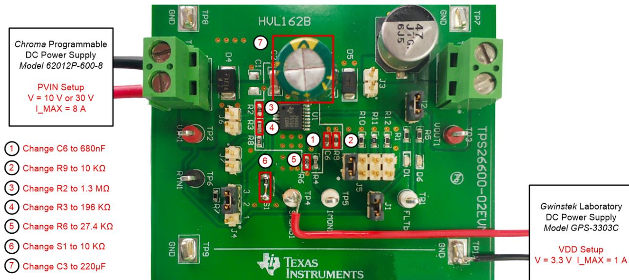
Figure 5-1. Bench Test Configuration of TPS26600 ASH PowerPath Management Application
