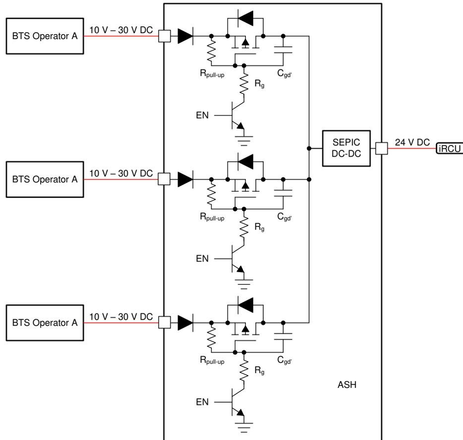
**Figure 2-2. Discrete Diodes and P-MOSFETs Solution for ASH PowerPath Management**
