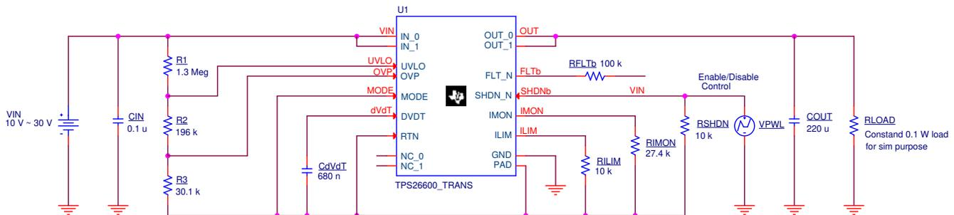
Figure 3-2. One Practical TPS26600 Circuit for ASH PowerPath Management
