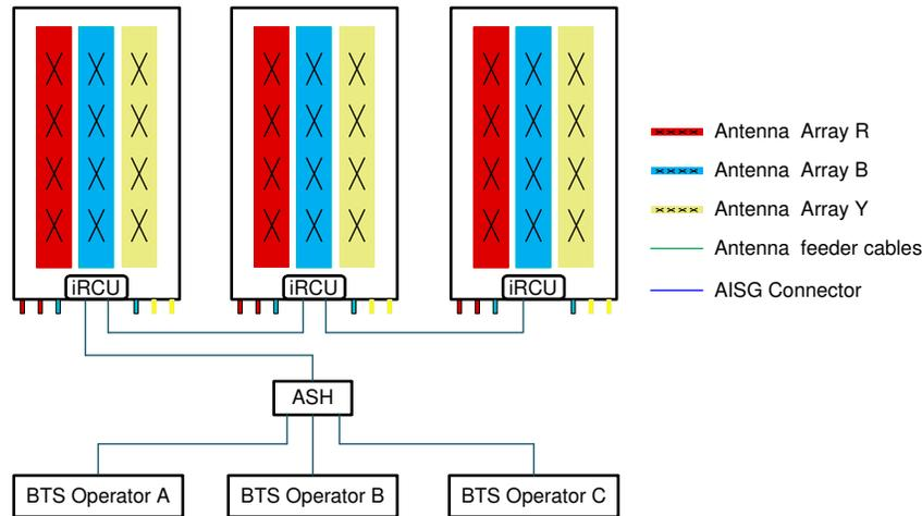
**Figure 1-2. Multi-band Antenna Deployment for Single Mode of Three Operators using ASH**
