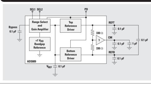
Figure 7. ADS809 internal reference circuit and recommended bypass scheme
