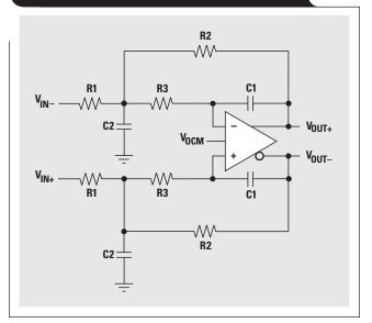
This is an active second-order low-pass filter, and the transfer function is
