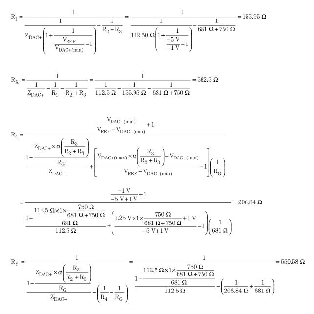
The nearest standard 1% values should be used:  $R_1$  = 154  $\Omega$ ,  $R_X$  = 562  $\Omega$ ,  $R_4$  = 205  $\Omega$ , and  $R_Y$  = 549  $\Omega$ .
