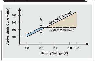
Figure 4 shows a battery-powered system that uses the TPS780xx to implement DVS to save battery power. The TPS780xx, which is an LDO with an ultralow quiescent current of 500 nA, contains a digital input ( $V_{SET}$ ) that connects directly to the MSP430. The MSP430 pulls this pin high to set  $V_{OUT}$  at 2.2 V and pulls it low to set  $V_{OUT}$  at 3.3 V. This configuration allows the MSP430 to adjust its input voltage as its operating conditions change.
