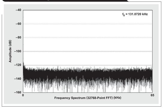
Figure 4 shows that the addition of  $R_1$  and  $C_3$  has a significant effect on the output noise for this system. The 9-kHz noise peak is gone. With this signal response, the output noise of the reference circuit in Figure 3 becomes  $2.2 \ \mu V_{RMS}$  or  $15 \ \mu V_{PP}$ , a reduction of nearly 90%. This improvement brings the noise level so well under control that the voltage-reference circuit is now appropriate for ADC resolutions of up to 20 bits.
