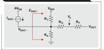
side to its minimum value,  $V_{DAC-} = V_{DAC-(min)}$ , and sets the DAC voltage on the positive side to its maximum value,  $V_{DAC+} = V_{DAC+(max)}$ . The value of  $1/R_4$  can then be used to find  $1/R_{Y}$ :
