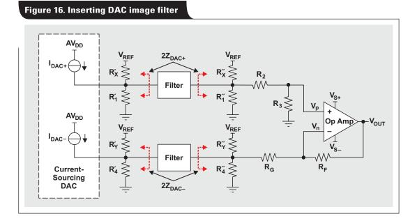
Figure 16 shows the proposed circuit implementation where  $R_1$ ,  $R_X$ ,  $R_4$ , and  $R_Y$  have been replaced with prime and double-prime components on either side of the filter, so that
