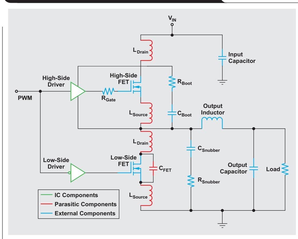
cycle, the converter prepares to switch the low-side FET off and the high-side FET back on to replenish power to the output L.
