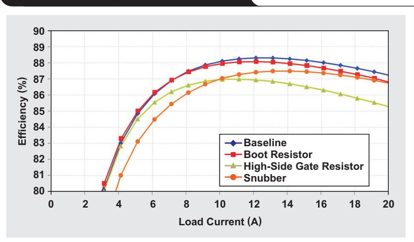
**Table 1. Test data for three methods of reducing ringing**
