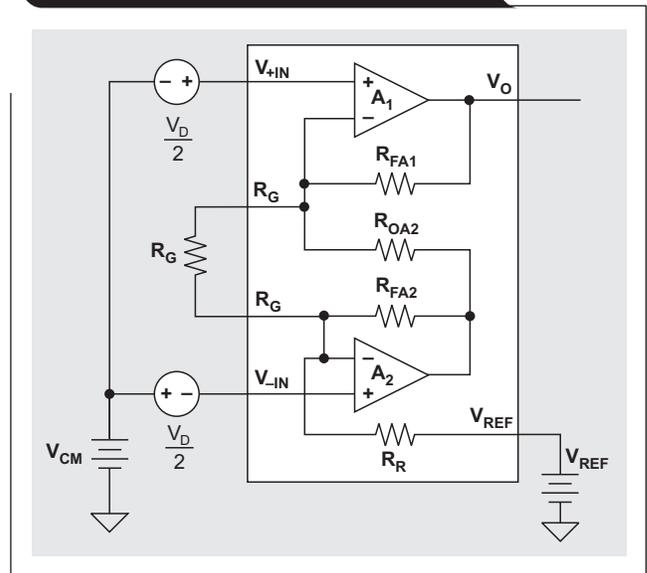
Figure 4. CMRR of two-op-amp vs. three-op-amp topologies
