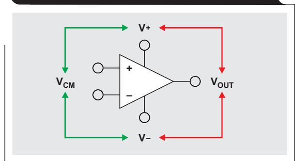
A real-world example of common-mode and output-swing limits is shown in Figure 8. Notice that the common-mode range and output-swing ranges are not necessarily the same.
