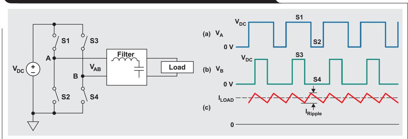
The instantaneous output power is  $V_{AB} \times I_{LOAD}$ , where  $V_{AB}$  is the average DC output, which is dependent on the duty cycles at nodes A and B. Assuming that there is no phase difference between the voltage and current, the output power for a sinusoidal output is:
