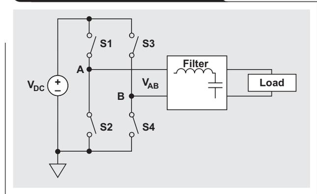
can range from 10 to 200 kHz, depending on the application and type of switch. In Figure 3a, the duty cycle at node A is more than 50% and in Figure 3b, the duty cycle is less than 50% at node B. This creates a positive voltage across the load as shown in Figure 3c.
