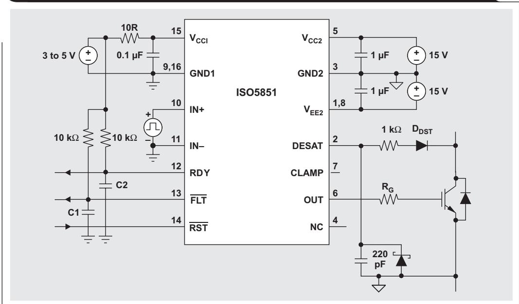
**Figure 8. Gate-driver solution using digital isolators**
