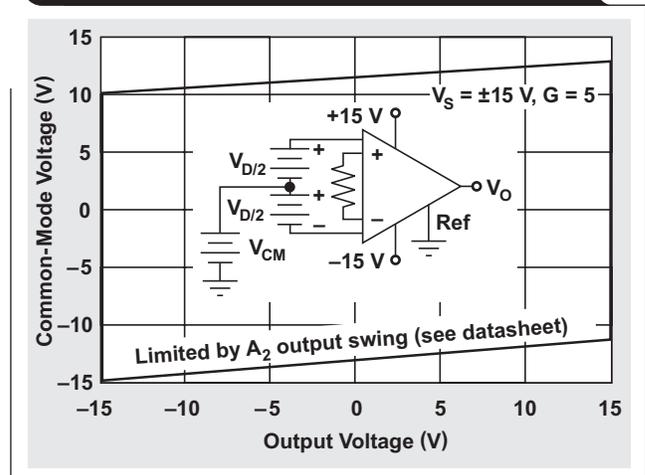
Figure 2. Instrumentation amplifier output distortion due to  $V_{CM}$  vs.  $V_{OUT}$  violation<sup>[1]</sup>
