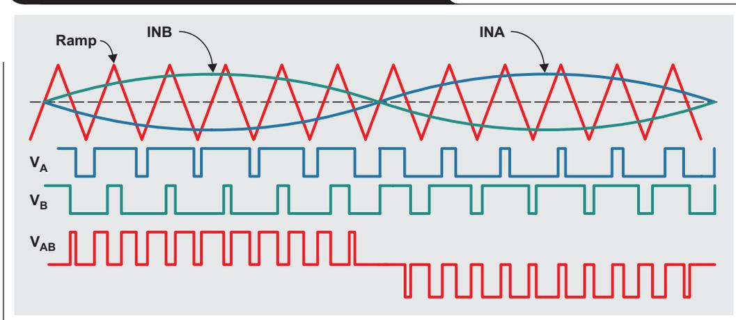
Controlling the duty cycle,  $D_A$  and  $D_B$ , allows control of the output voltage,  $V_{AB}$ . A sinusoidal single-phase PWM waveform is obtained by comparing a reference sine wave  $INA$  and  $INB$  with a high-frequency triangular signal as shown in Figure 4.
