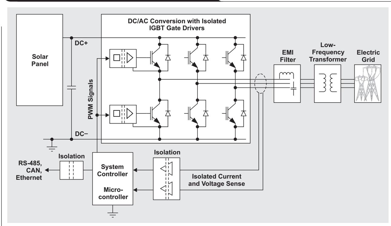
isolated gate drivers or isolators passing gate controls to power transistors see large ground transients because one ground is connected to rapidly switching inverter outputs. Figure 5 shows the ground potential difference experienced by these gate drivers. In these systems, CMTI is a critical parameter because any bit errors caused by the transients can result in dangerous short-circuit events.
