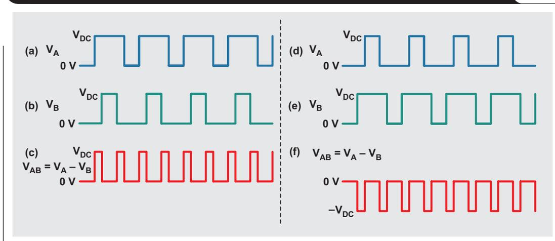
Figure 4. A single-phase PWM output waveform
