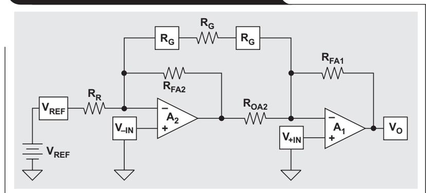
The gain applied to the instrumentation amplifier's reference voltage should be 1 V/V. To fulfill this requirement, set  $R_{FA1} = R_R$  and  $R_{FA2} = R_{OA2} = R_F$ . Figure 6 depicts the updated two-op-amp topology that results in unity gain for the reference voltage. Furthermore, the internal nodes are labeled for future analysis.
