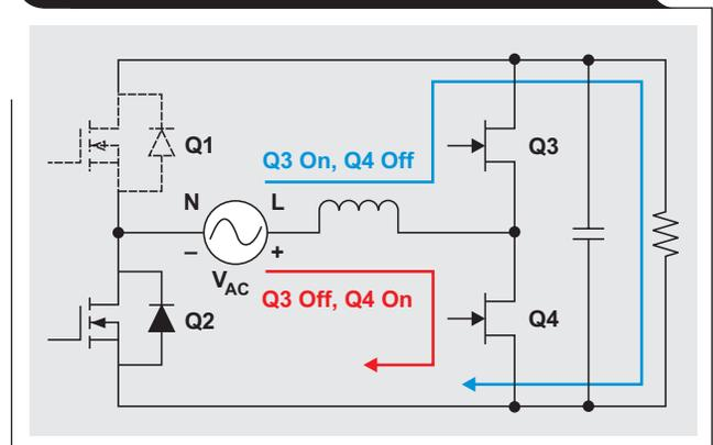
**Figure 4. Current paths for negative AC cycle**
