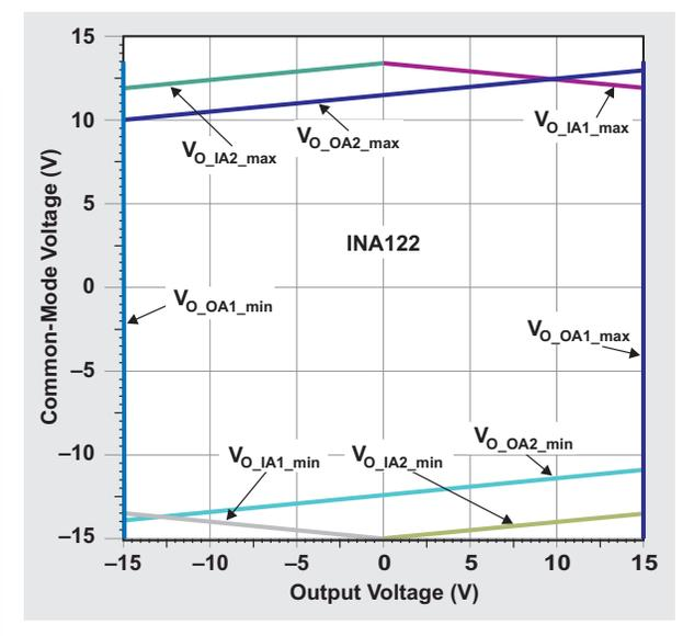
Figure 10.  $V_{CM}$  vs.  $V_{OUT}$  software tool
