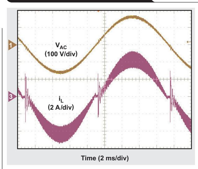
Figure 9. Current waveform with the proposed control method
