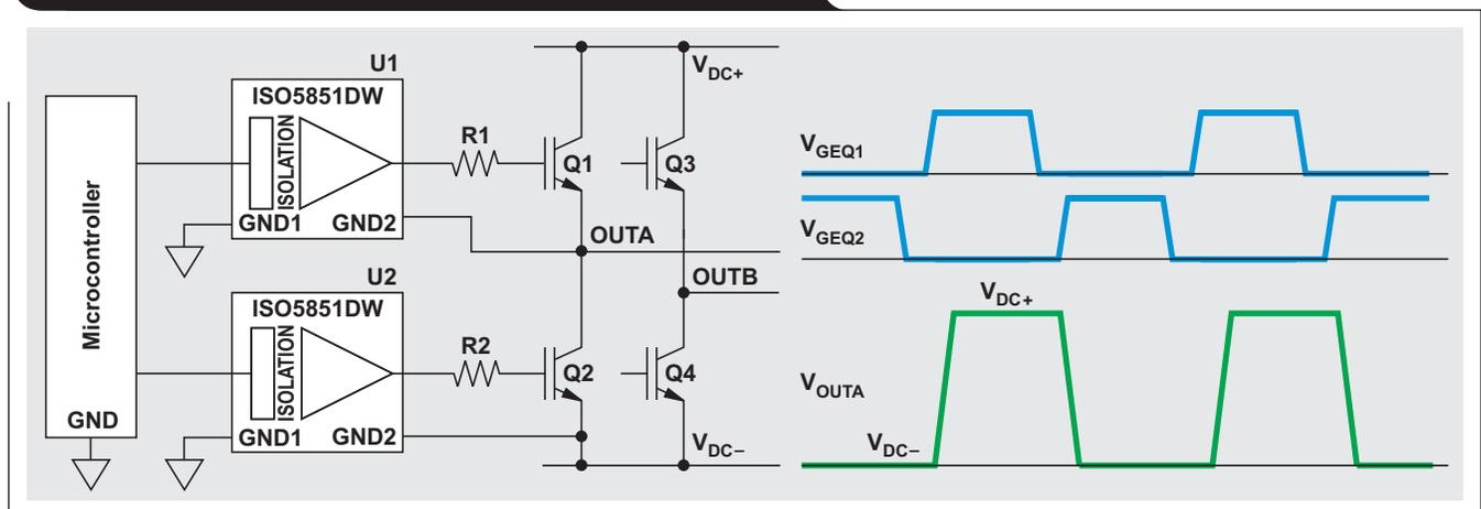
ISO5851 datasheet, Figure 7 shows a typical application diagram. The Ready (RDY) and Fault (FLT) pins are pulled up by 10-kΩ resistors. These resistor values may need to be lower for noise immunity. Transient noise can generate a false fault or low under-voltage lockout (UVLO) signal. This issue can be solved by either reducing the resistor values or increasing the capacitance of C1 and C2.
