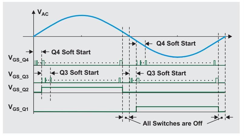
this dead zone. Otherwise, when the PFC turns back on, the integrator build-up in the loop generates a large PWM pulse, which can cause a large current spike.
