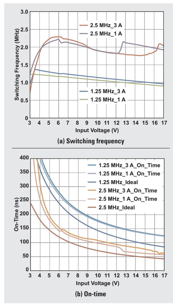
current capability. High-frequency operation is maintained for the common applications of USB ports and system rails with higher voltages.
