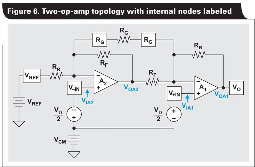
Figure 6. Two-op-amp topology with internal nodes labeled
