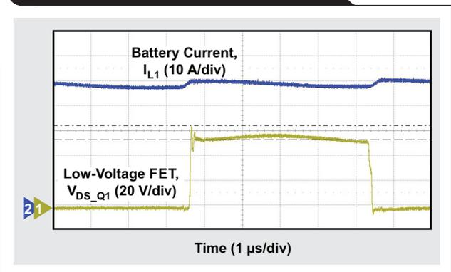
Figure 6. Active-clamp waveforms
