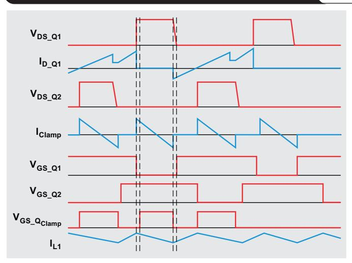
Figure 5. Low-voltage MOSFET  $V_{DS}$  and inductor current
