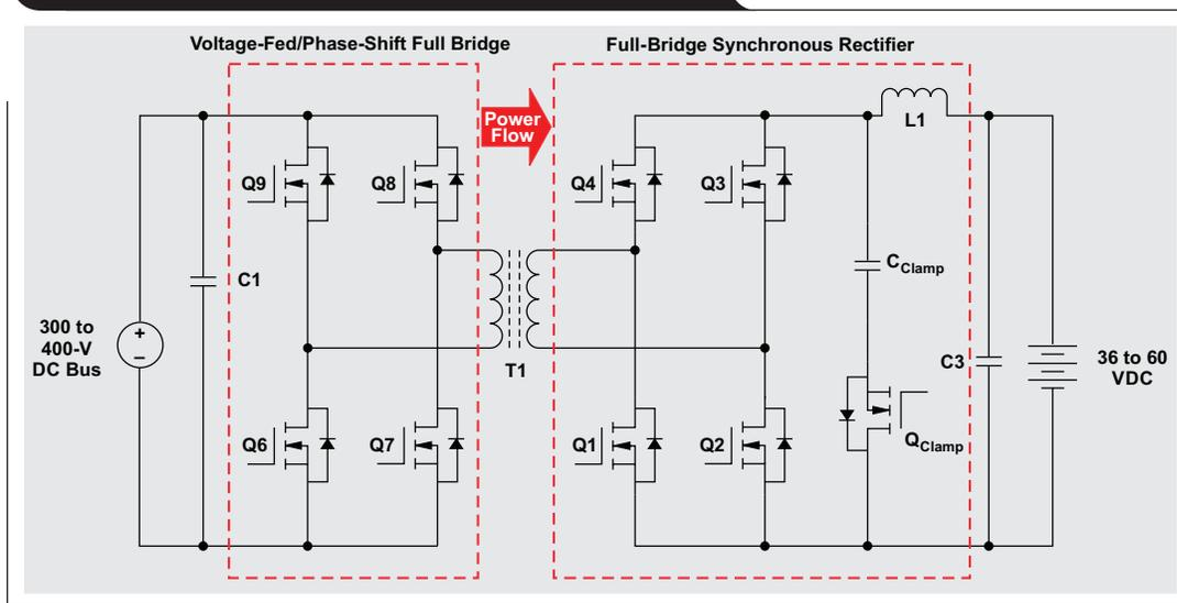
**Figure 3. Active-clamp current-fed full-bridge backup supply**
