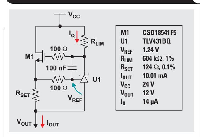
**Table 3. Current-source specifications using a shunt regulator**
