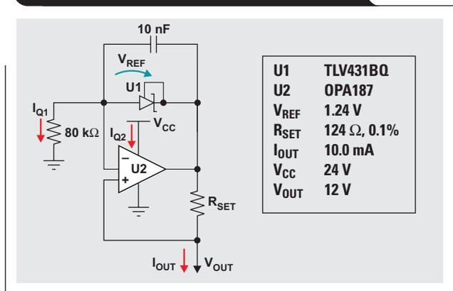
**Table 4. Current-source specifications using a shunt regulator and op amp**
