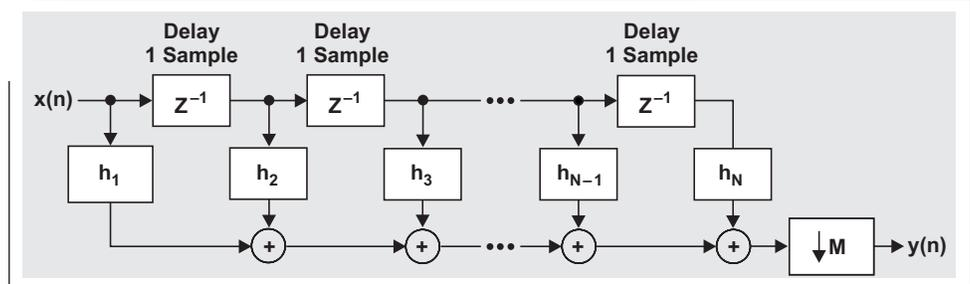
Figure 4. Block diagram of a complex decimation filter
