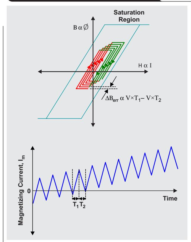
**Figure 4. Current limiting prevents  $I_m$  from building up to unsafe levels**
