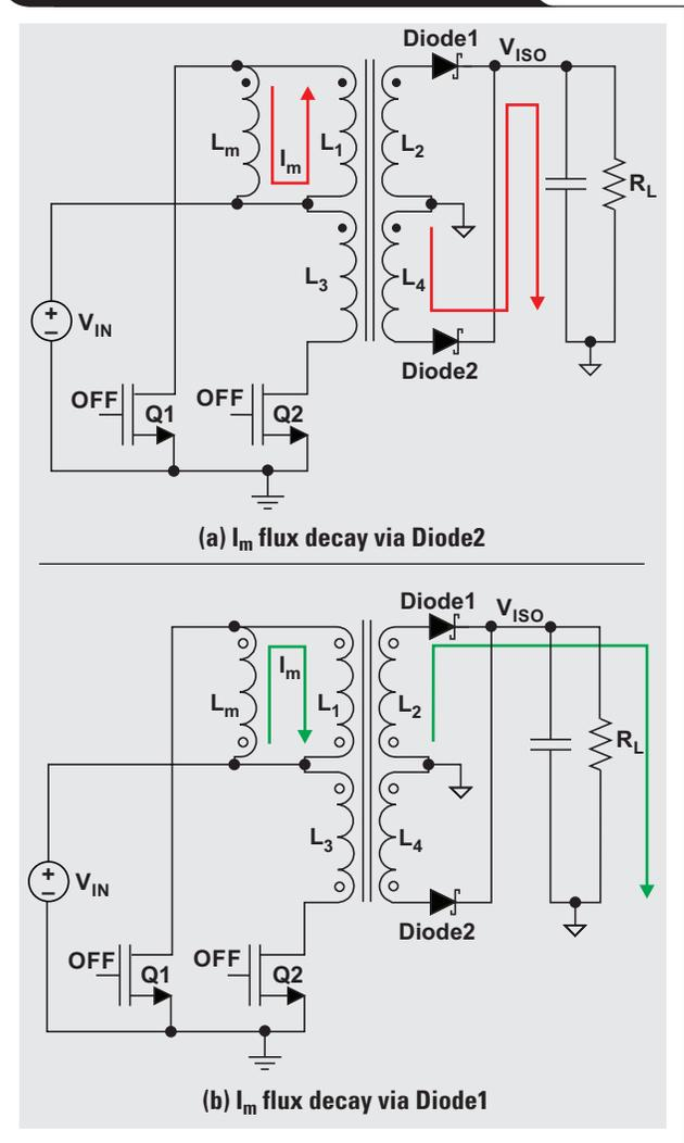
Figure 6. Flux and  $I_m$  remain stable in spite of a mismatch, decaying to zero during dead time (DT)
