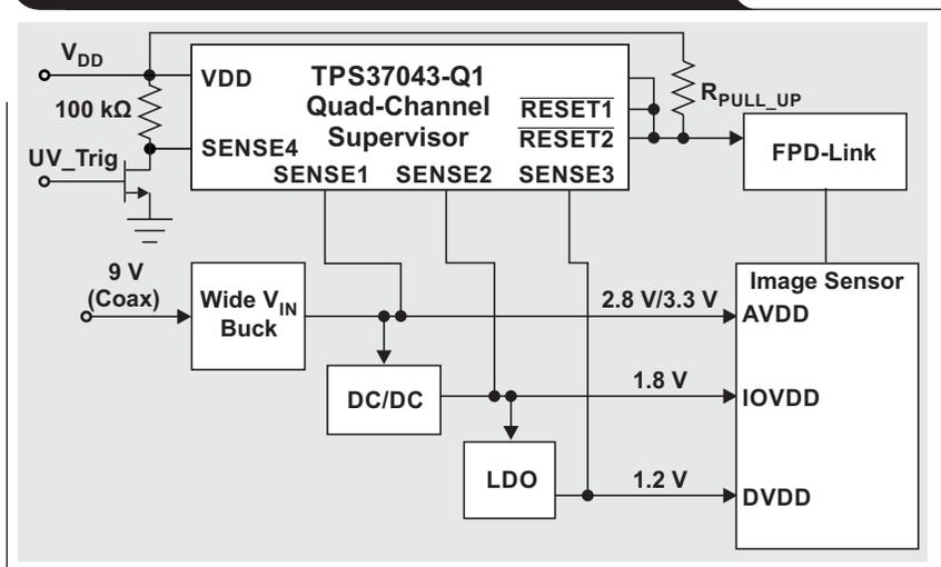
Figure 3. Manual check of over- and undervoltage trip points
