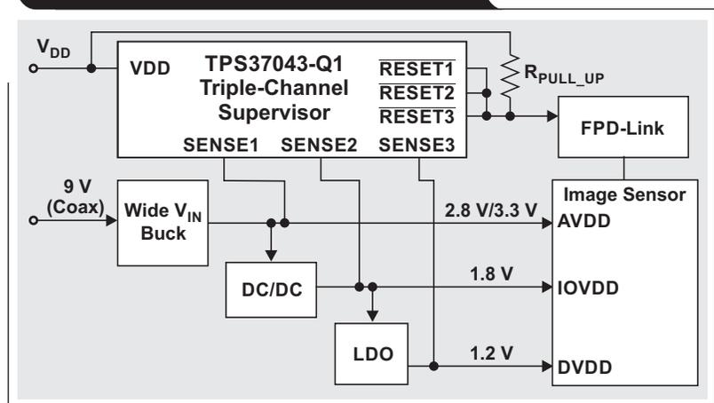
job of the voltage supervisor in this case is to cause a reset of the image sensor if a hung state occurs so that the system reboots.
