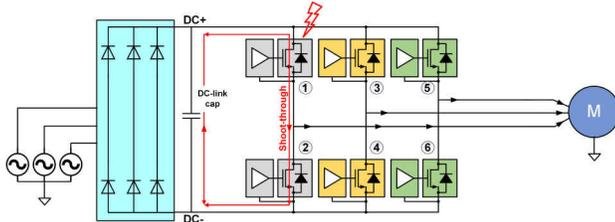
**Figure 2.** A shoot-through fault in electric motor drives.
