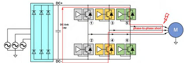
**Figure 4.** A phase-to-phase short in electric motor drives.
