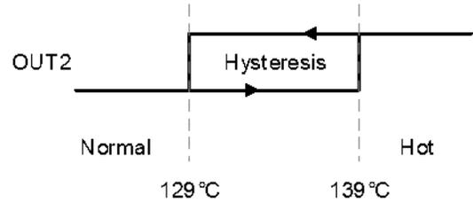
Figure 13. AMC23C14 output waveform.
