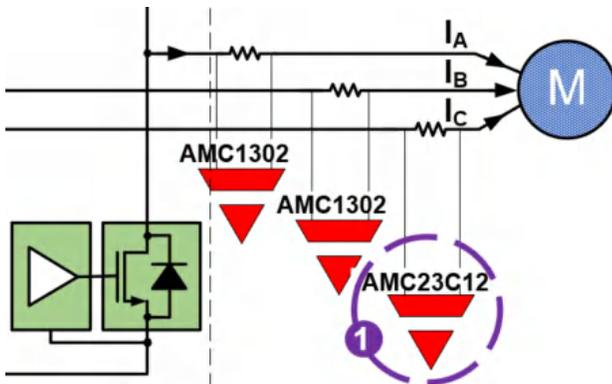
**Figure 6.** Bidirectional in-phase overcurrent detection.
