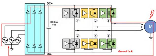
**Figure 3.** A ground fault in electric motor drives.
