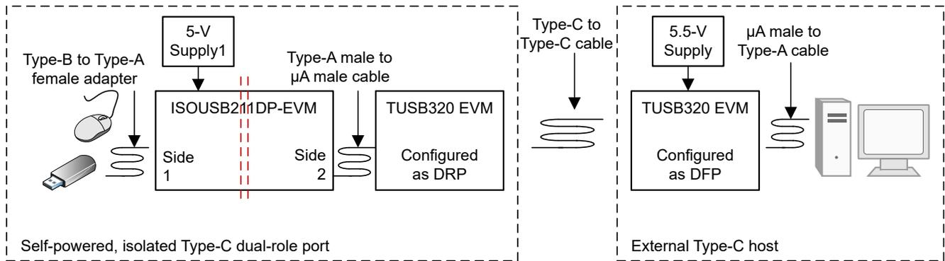
**Figure 6.** The ISOUSB211 and TUSB320 as a DRP connected to a USB Type-C host
