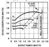
FIGURE 3a. Device Dissipation vs Output Power —  $4\Omega$  Load
