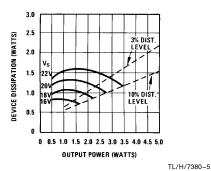
FIGURE 3c. Device Dissipation vs Output Power —  $16\Omega$  Load
