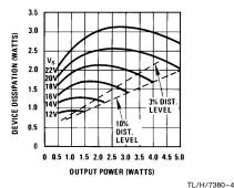
FIGURE 3b. Device Dissipation vs Output Power — 8 $\Omega$  Load
