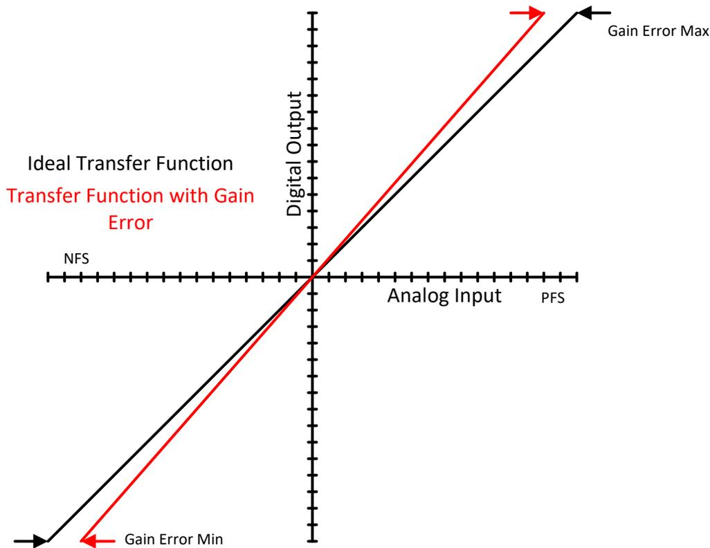
Figure 4-1. ADC Input to Output With Gain Error
