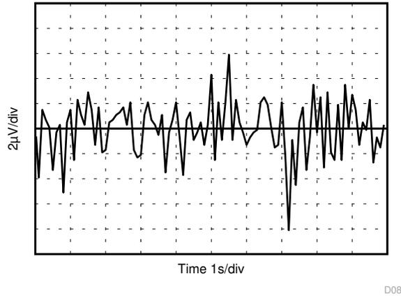
**Figure 6-2. REF3425 0.1Hz to 10Hz Noise**
