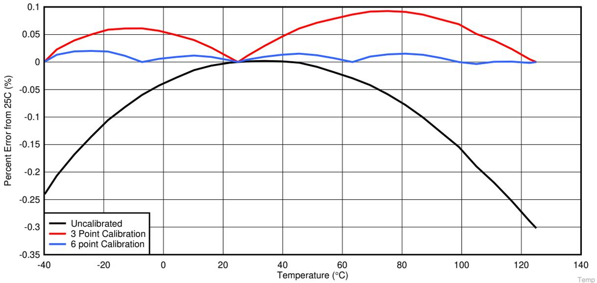
**Figure 5-1. Temperature Drift Error With Calibration Profiles**
