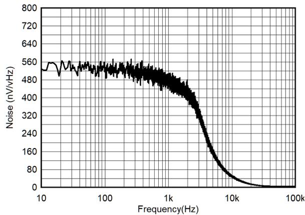
**Figure 6-3. REF3425 Noise Performance 10Hz to 100kHz**
