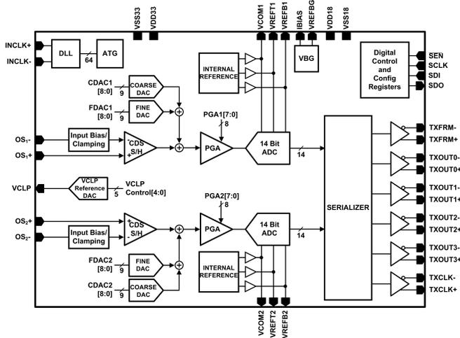
Figure 2. LM98640 Block Diagram
