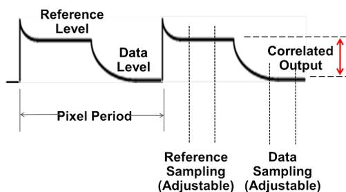
**Figure 1. CCD Output and Correlated Doubling Sampling**
