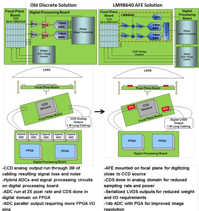
Figure 3. Discrete Solution vs AFE Solution
