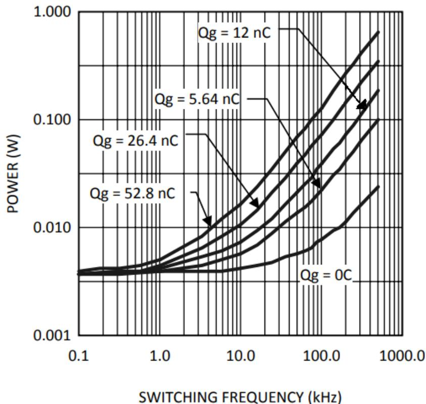
**Figure 2. Gate -Driver Power Dissipation (LO and HO)**
