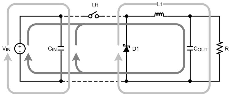
Figure 3. High-Current Paths of a Buck Regulator
