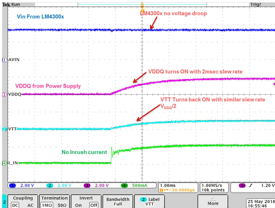
Figure 7. Inrush Current Controlled by RC Filter
