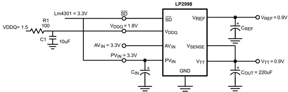
Figure 6. Inrush Current Controlled by RC Filter
