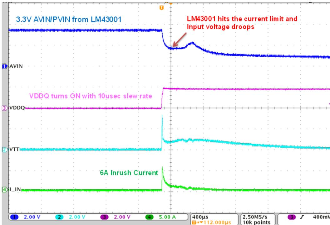
Figure 3. System Shutdown Due to Inrush Current
