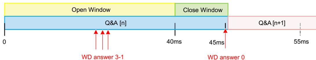
**Figure 3. WDT Response Timing in the Examples**
