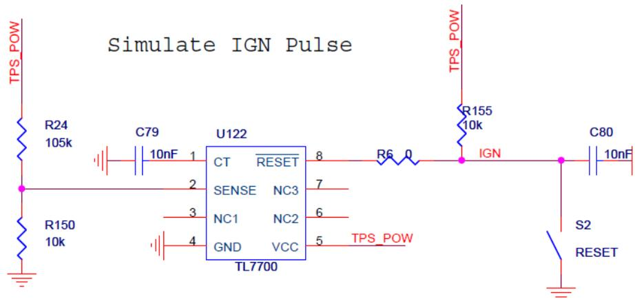
**Figure 2. Circuit to Simulate the IGN Pulse**
