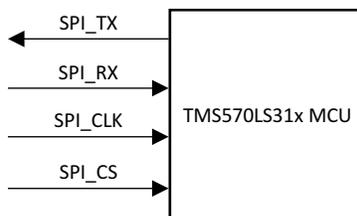
**Figure 1. SPI Connections for TMS570LS31x Bootloader**
