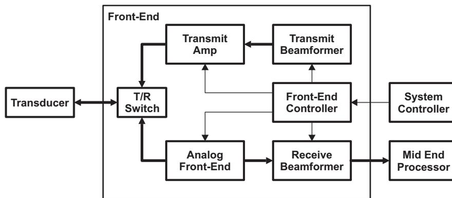
Figure 2. Components of Front-End Processing
