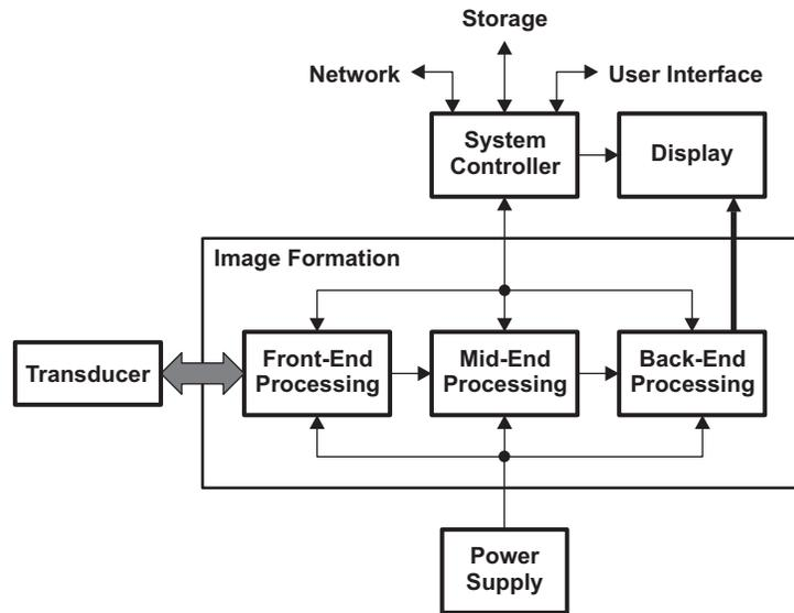
Figure 1. Ultrasound Imaging System Functional Blocks
