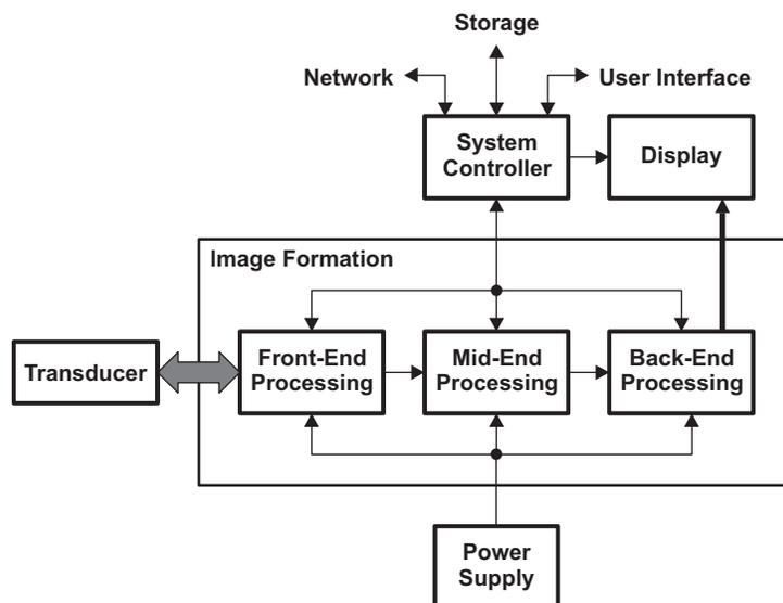
Figure 1. Ultrasound Imaging System Functional Blocks
