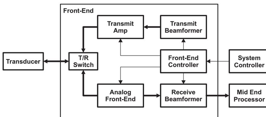
Figure 2. Components of Front-End Processing
