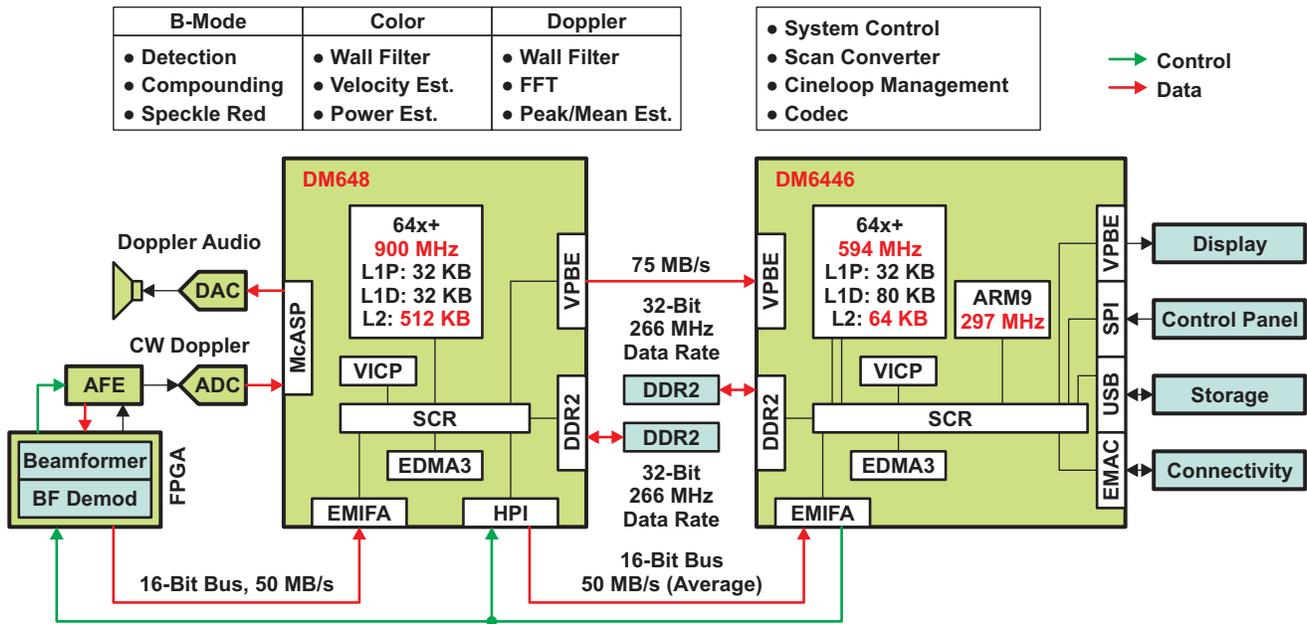
Figure 5. DM648 + DM6446 Block Diagram
