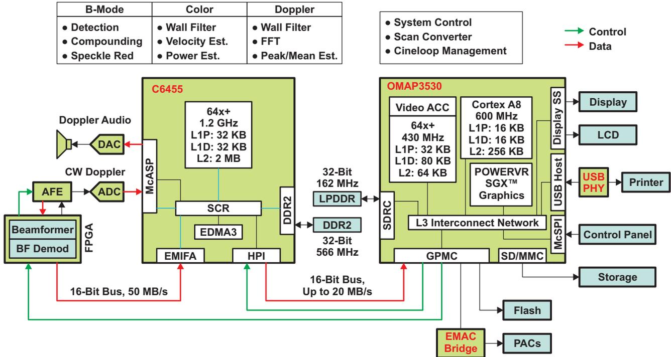
Figure 6. C6455 + OMAP3530 Block Diagram
