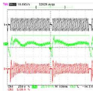
Figure 16. With Anti-Integral Windup
