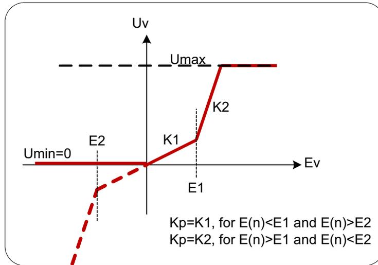
**Figure 10. Non-Linear Control of PFC**
