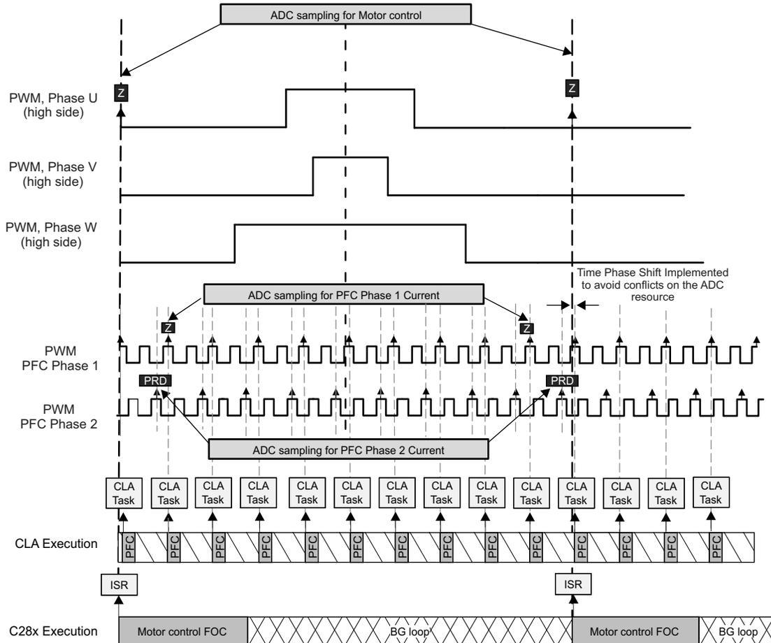
**Figure 6. PFC Implemented on the CLA and Motor Control on C28x**
