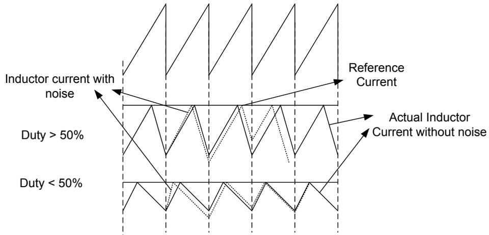
**Figure 2. Noise Changes in Different Duty Cycle**
