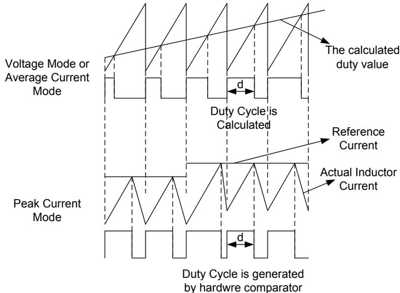
**Figure 1. PWM Generation in Peak Current Mode**
