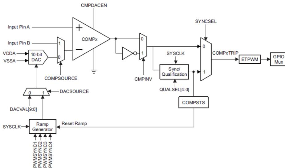
**Figure 4. Block Diagram of the Internal Comparator**
