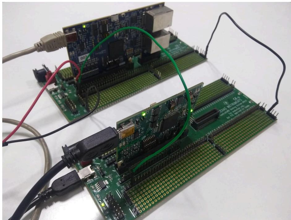
**Figure 4. Test Setup for Cross Device Data Transfer**
