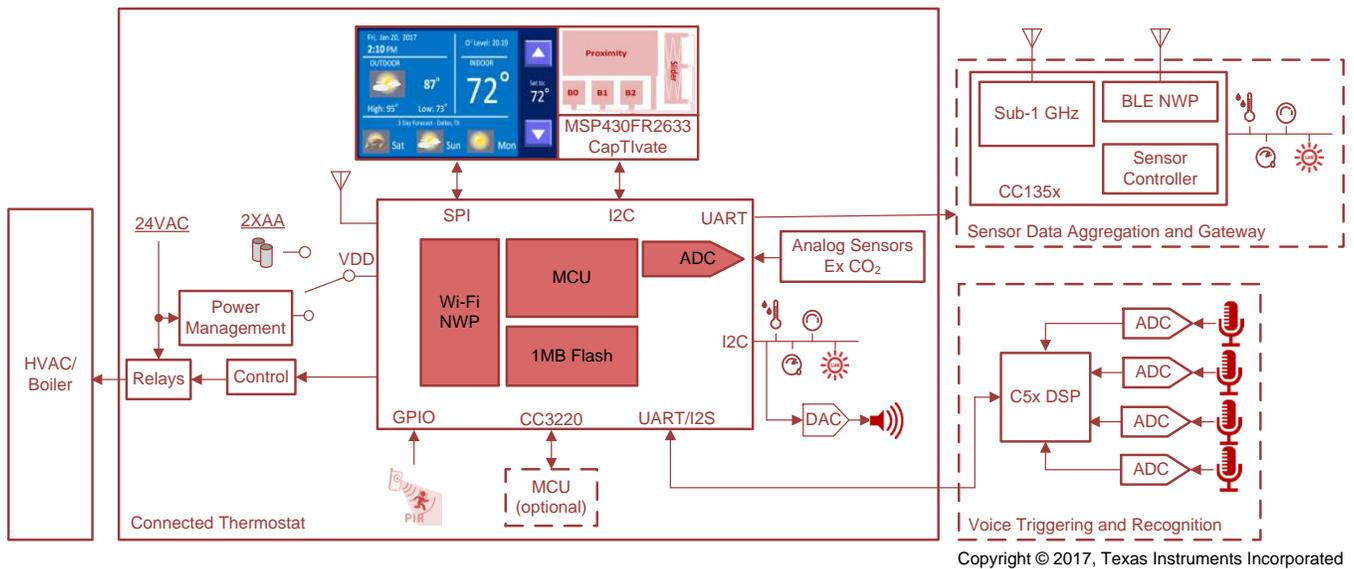
**Figure 2. Block Diagram of the Thermostat Design Based on CC3220 Wi-Fi and MCU SoC**
