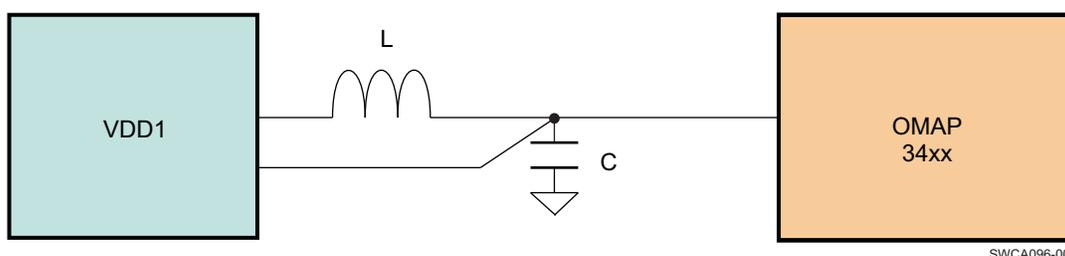
**Figure 1. VDD1 External Components Connectivity for OMAP34xx**
