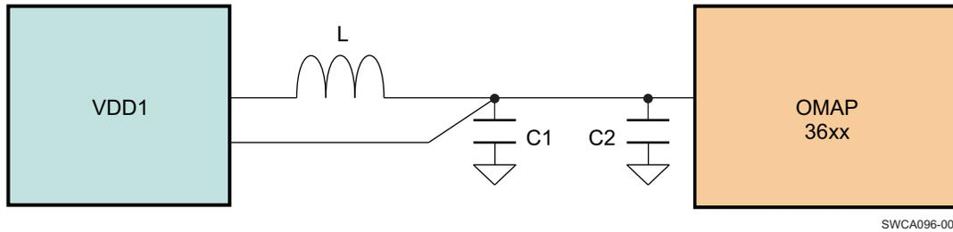
Figure 2. VDD1 External Components Connectivity for OMAP36xx
