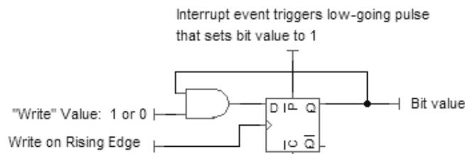
Figure 2. Simplified Write-0 Bit Model
