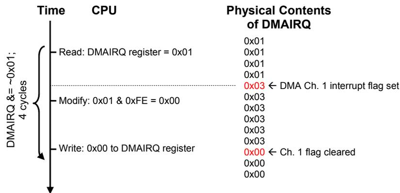
**Figure 1. Timing diagram showing a missed interrupt flag on DMA channel 1 due to the instruction, `DMAIRQ &= ~0x01`, to clear the DMA channel 0 interrupt flag.**
