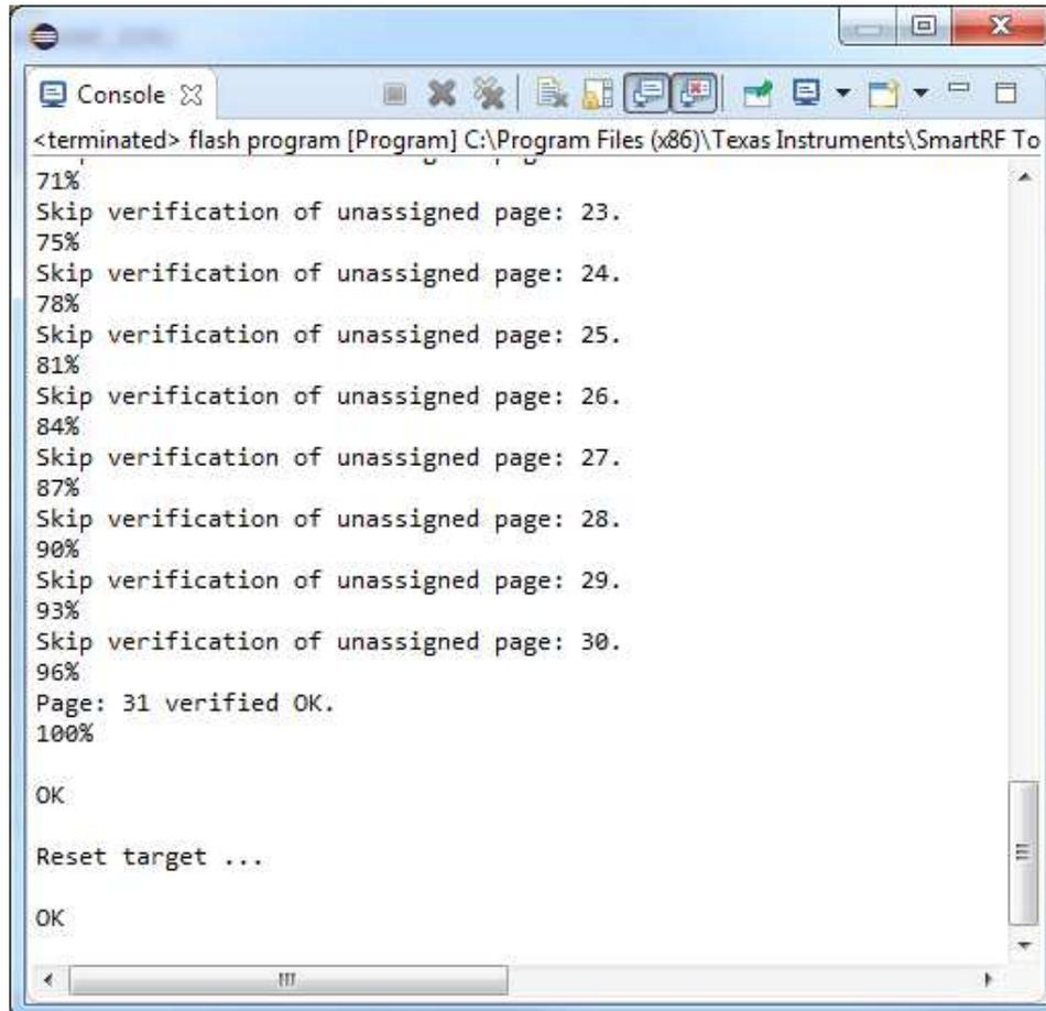
**Figure 18. Load the Image to Target (Windows)**
