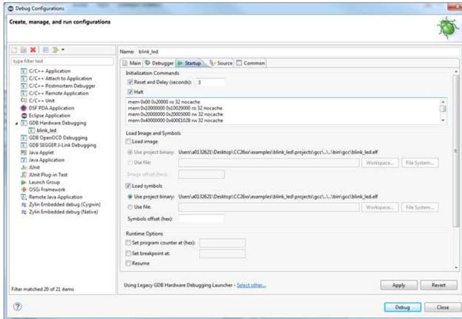
Figure 24. GDB Hardware Debugging – Startup Tab
