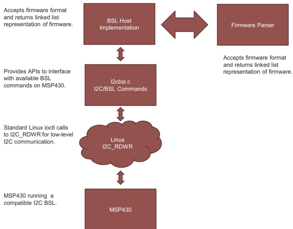
Figure 1. Overall I²C BSL Update Block Diagram
