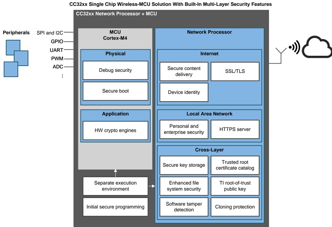
**Figure 3. CC3220/CC3235x Device Security Features**
