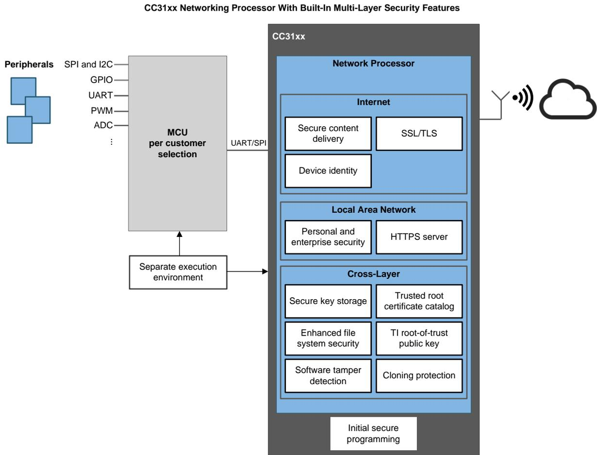
**Figure 4. CC3120/CC3135 Device Security Features**
