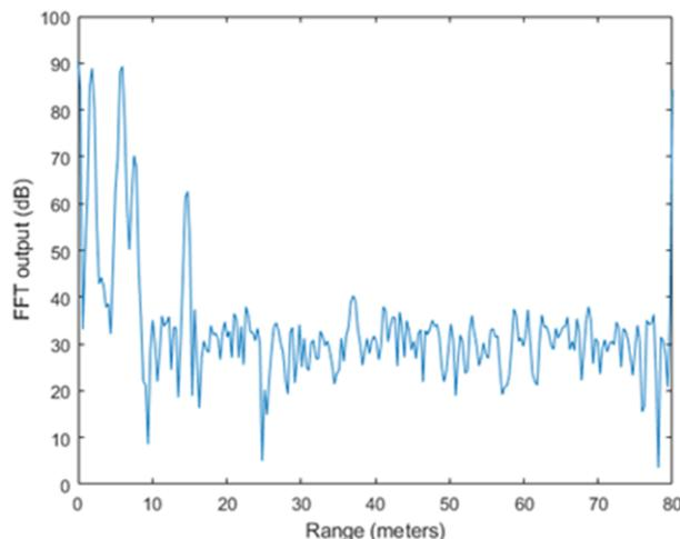
**Figure 4. Typical Range FFT Output**
