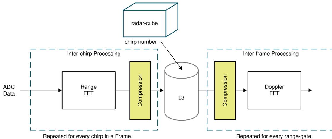
**Figure 3. Standard Radar Processing Flow**
