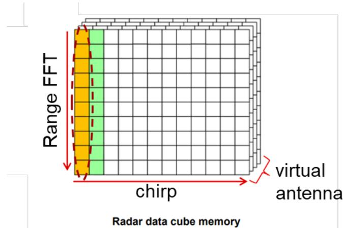
Figure 1. A Typical Radar Cube
