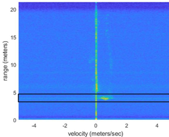
Figure 7. Range-Doppler Image for a 33% Compressed Radar Cube
