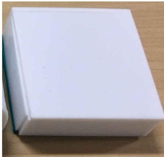
**Figure 6-4. PTFE-Based Rectangular Radome With 1.524 mm Wall Thickness**
