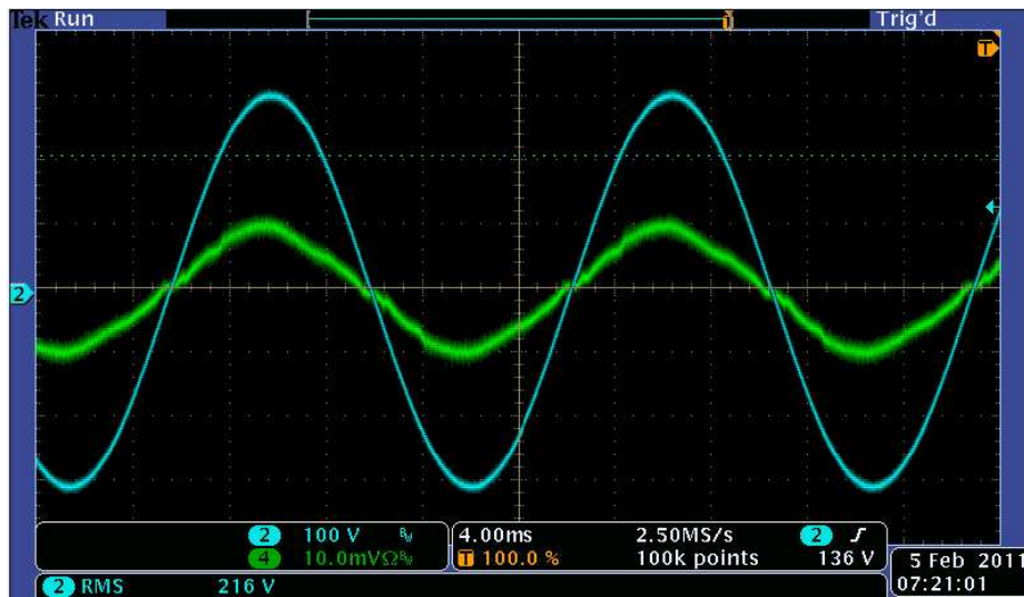
Figure 17. BL PFC Input Voltage and Current Waveforms (Pout = 300W)
