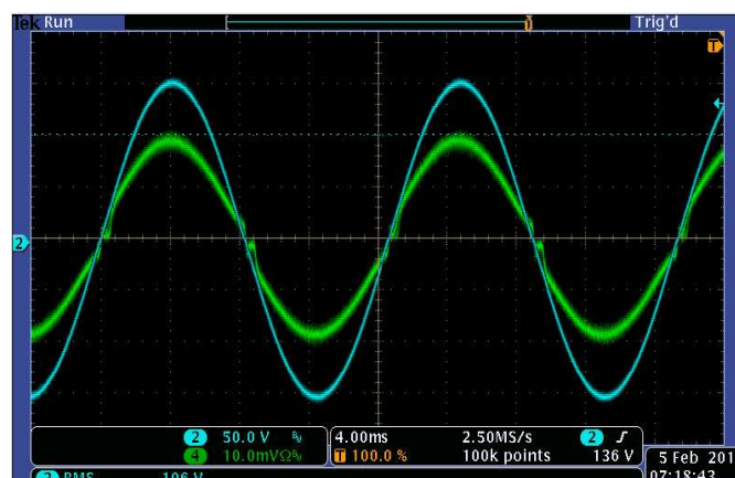
Figure 16. BL PFC Input Voltage and Current Waveforms at 150W
