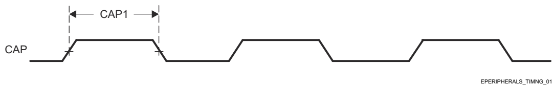
図 6-29. ECAP Timings Requirements
