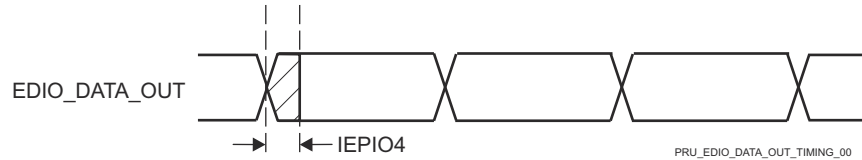
図 6-100. PRU_ICSSG IEP Digital IOs Timing Requirements
