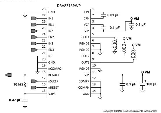
Figure 17. Three Independent Load Connections Schematic
