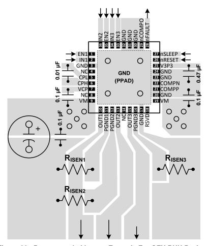
Figure 20. Recommended Layout Example For QFN RHH Package
