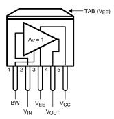
The KTT package is non-isolated package. The package's metal back and any heat sink to which it is mounted are connected to the same potential as the  $-V_{\text{EE}}$  pin.
