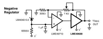
Figure 31. High Speed Positive and Negative Regulator
