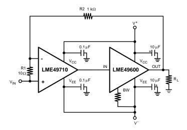
Figure 27. THD+N Distortion Test Circuit
