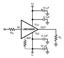
Figure 29. Buffer Connections
