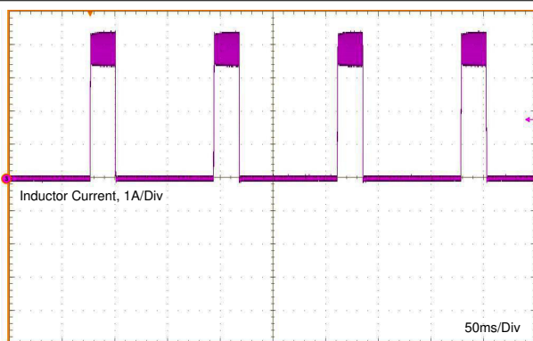
図 8-5. Inductor Current Burst in Short-Circuit Mode
