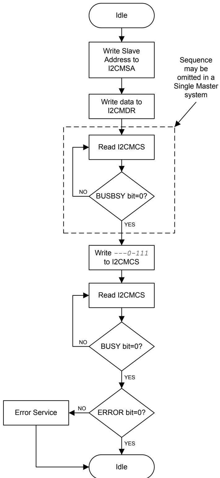
**Figure 21-9. Master Single RECEIVE**
