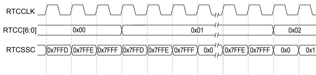
In the case of a trim value below 0x7FFF, the RTCSSC value is advanced from 0x7FFF to the trim value while the RTCC value is incremented from 0x0 to 0x1. If the match value is within that range, the match interrupt is not triggered. For example, as shown in Figure 7-6 on page 550, if the match interrupt was configured with RTCM0=0x1 and RTCSSM=0x2, an interrupt would never be triggered.
