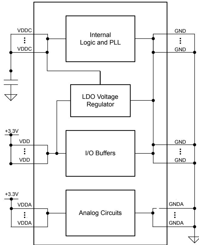
**Note:** The V<sub>DDA</sub> voltage source is typically connected to a filtered voltage source or regulator.
