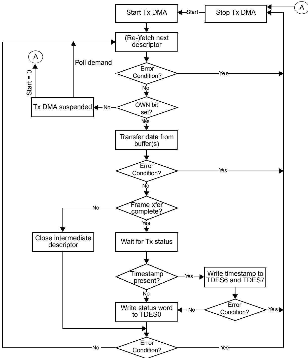
***TX DMA OSF Mode Operation***
