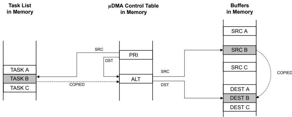
Using the channel's primary control structure, the μDMA controller copies task B configuration to the channel's alternate control structure.
