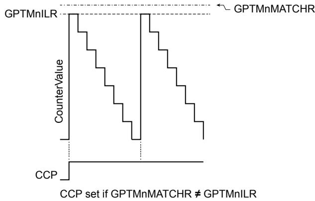
Figure 16-6 on page 1092 shows how the CCP output operates when the **PLO** and **MRSU** bits are set and the **GPTMTnMATCHR** value is the same as the **GPTMTnILR** value. In this situation, if the **PLO** bit is 0, the CCP signal goes high when the **GPTMTnILR** value is loaded and the match would be essentially ignored.
