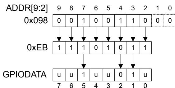
During a read, if the address bit associated with the data bit is set, the value is read. If the address bit associated with the data bit is cleared, the data bit is read as a zero, regardless of its actual value. For example, reading address GPIO DATA + 0x0C4 yields as shown in Figure 10-4. This example shows how to read **GPIODATA** bits 5, 4, and 0.
