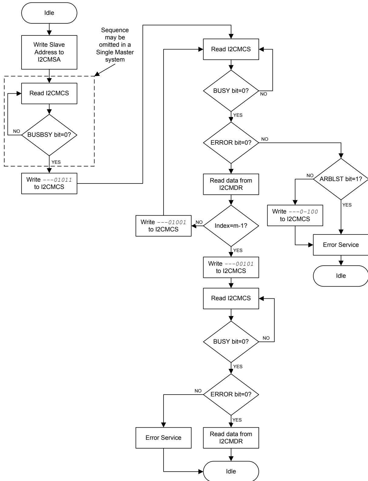
**Figure 21-12. Master RECEIVE with Repeated START after Master TRANSMIT**
