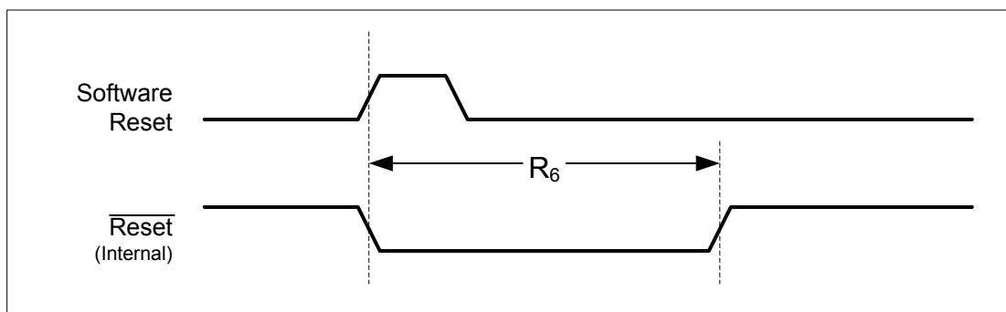
**Figure 30-13. Watchdog Reset Timing**
