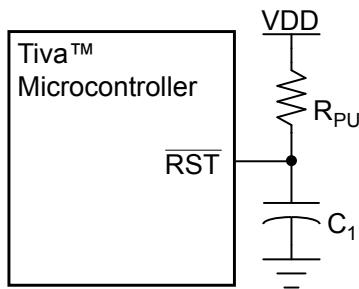
**Note:**  $R_{PU} = 1\text{ k}\Omega$  to  $100\text{ k}\Omega$
