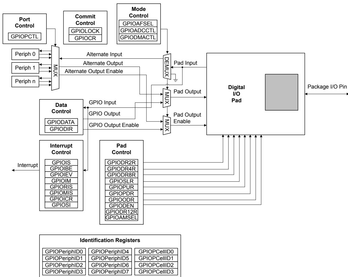
**Figure 10-2. Analog/Digital I/O Pads**
