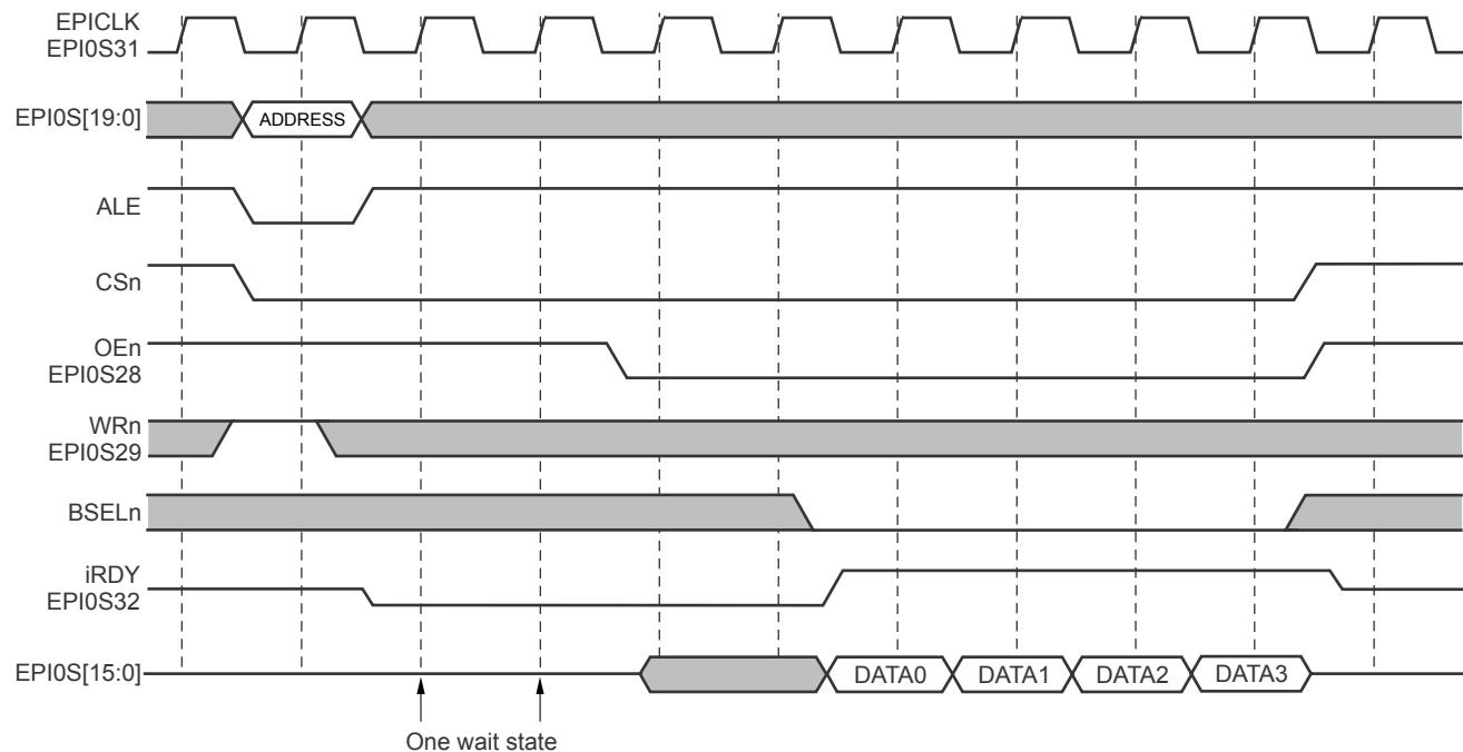
**Figure 11-10. Write Delay During Refresh Event**
