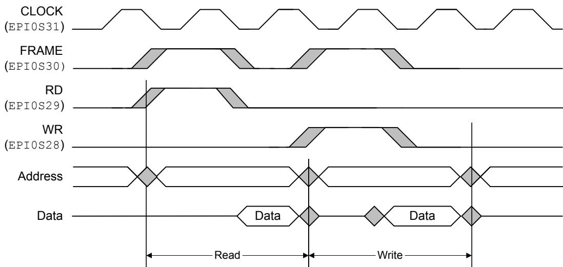
**Figure 11-21. Read Accesses, FRM50=0, FRMCNT=0**
