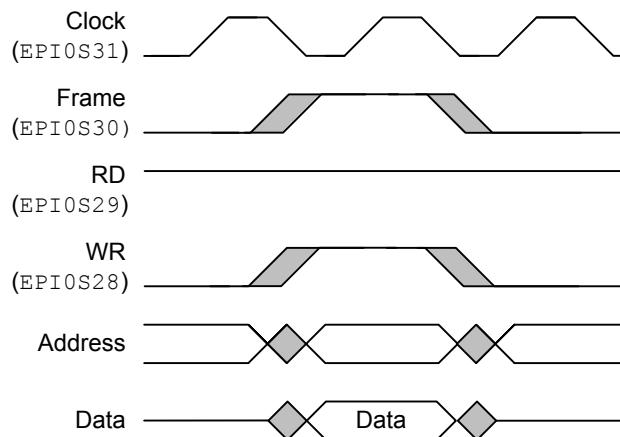
**Figure 11-20. Two-Cycle Read, Write Accesses, FRM50=0, FRMCNT=0, WR2CYC=1**
