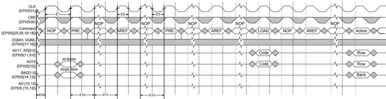
**Figure 30-19. SDRAM Read Timing**
