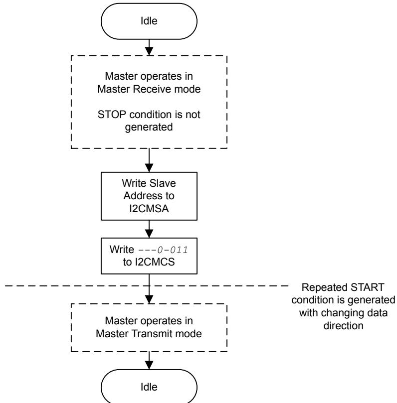
Figure 21-14. Standard High Speed Mode Master Transmit
