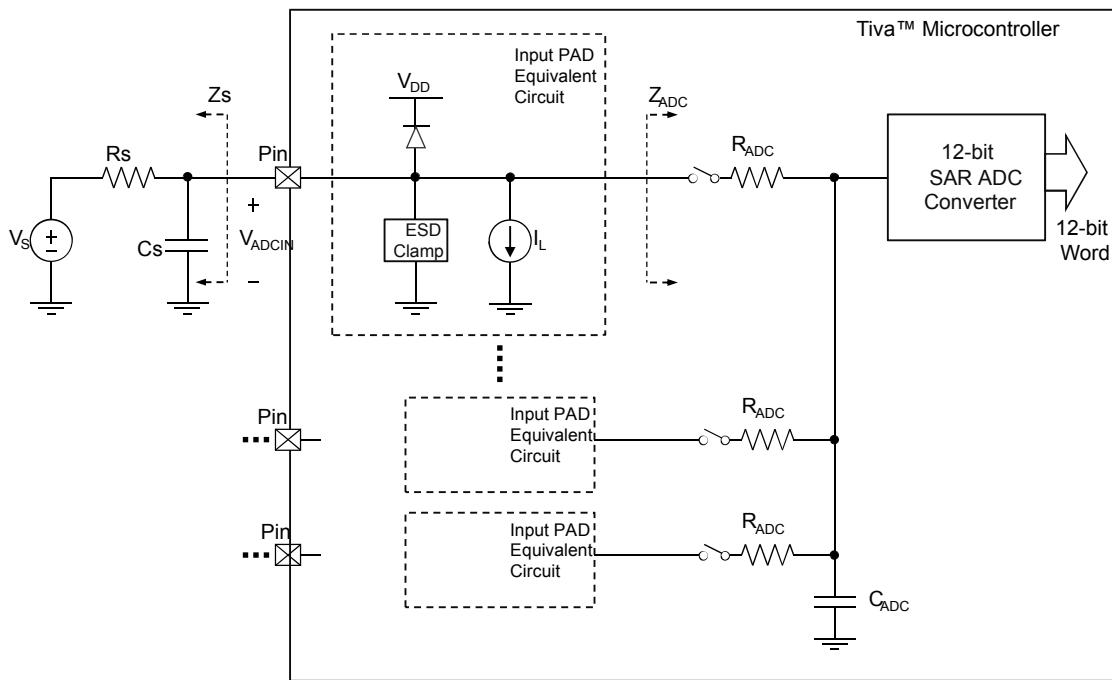
The ADC operates from both the 3.3-V analog and 1.2-V digital power supplies. The ADC clock can be configured to reduce power consumption when ADC conversions are not required (see “System Control” on page 246). The analog inputs are connected to the ADC through specially balanced input paths to minimize the distortion and cross-talk on the inputs. Detailed information on the ADC power supplies and analog inputs can be found in “Analog-to-Digital Converter (ADC)” on page 1985.
