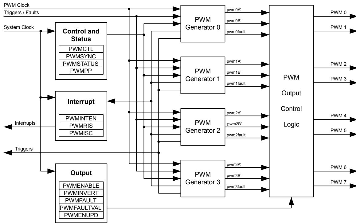
**Figure 26-2. PWM Generator Block Diagram**
