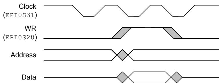
**Figure 11-29. EPI Clock Operation, CLKGATE=1, WR2CYC=1**
