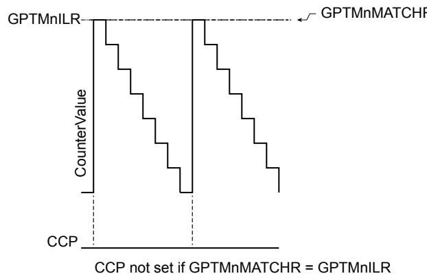
Figure 16-7 on page 1092 shows how the CCP output operates when the **PLO** and **MRSU** bits are set and the **GPTMTnILR** is greater than the **GPTMTnMATCHR** value.
