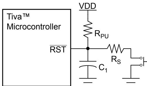
**Note:** Typical  $R_{PU} = 10\text{ k}\Omega$
