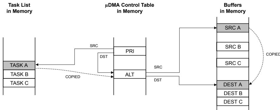
Using the channel's primary control structure, the μDMA controller copies task A configuration to the channel's alternate control structure.
