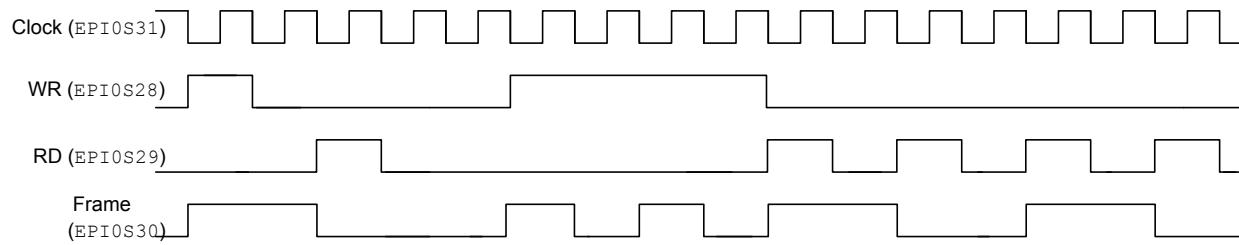
When FRMCNT=1, the FRAME signal transitions on the rising edge of the WR or RD strobes for every other access, see Figure 11-26 on page 861.
