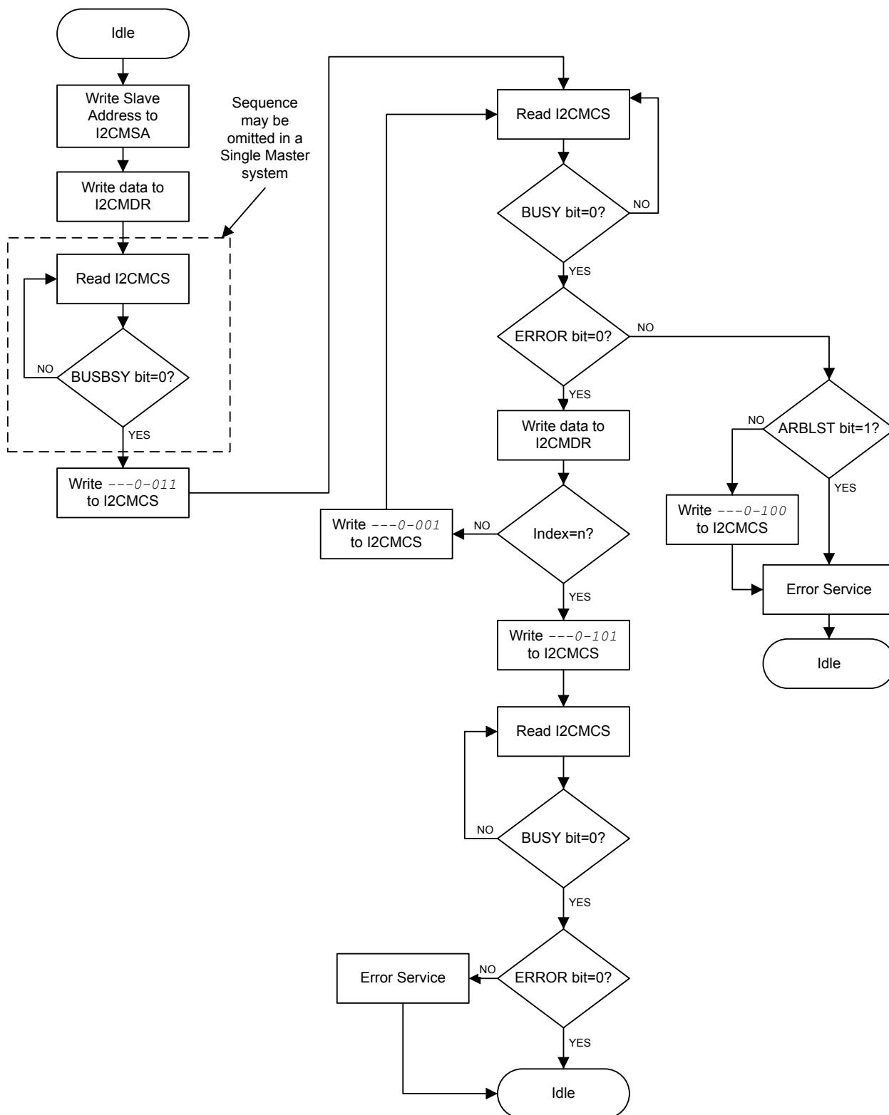
**Figure 21-11. Master RECEIVE of Multiple Data Bytes**
