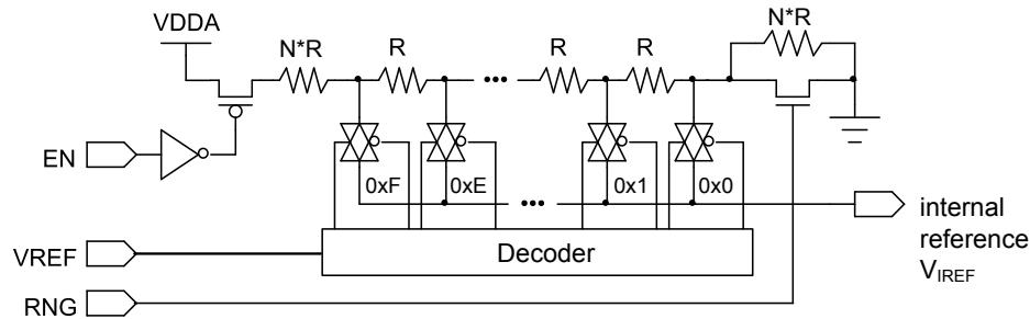
**Note:** In the figure above,  $N^*R$  represents a multiple of the  $R$  value that produces the results specified in Table 25-2 on page 1780.
