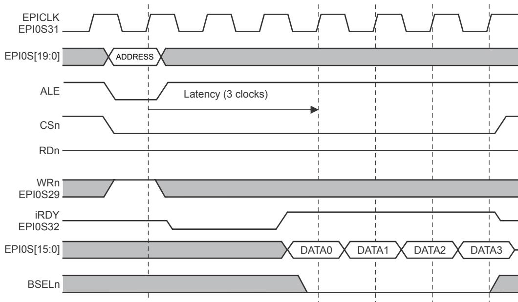
**Figure 11-8. PSRAM Burst Write**
