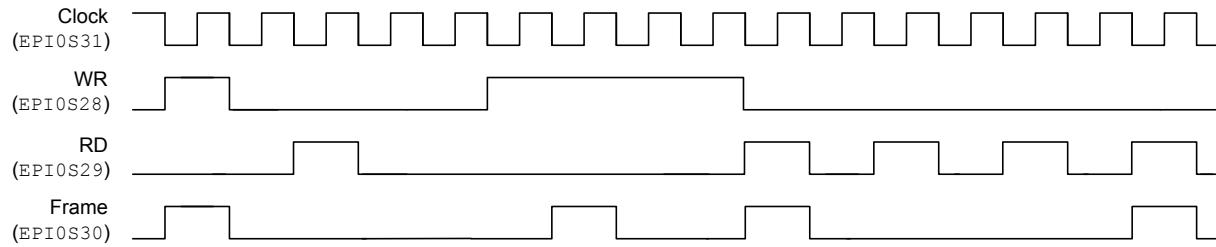
When FRM50 is set, the FRAME signal transitions on the rising edge of either the WR or RD strobes. When FRMCNT=0, the FRAME signal transitions on the rising edge of WR or RD for every access, see Figure 11-25 on page 860.
