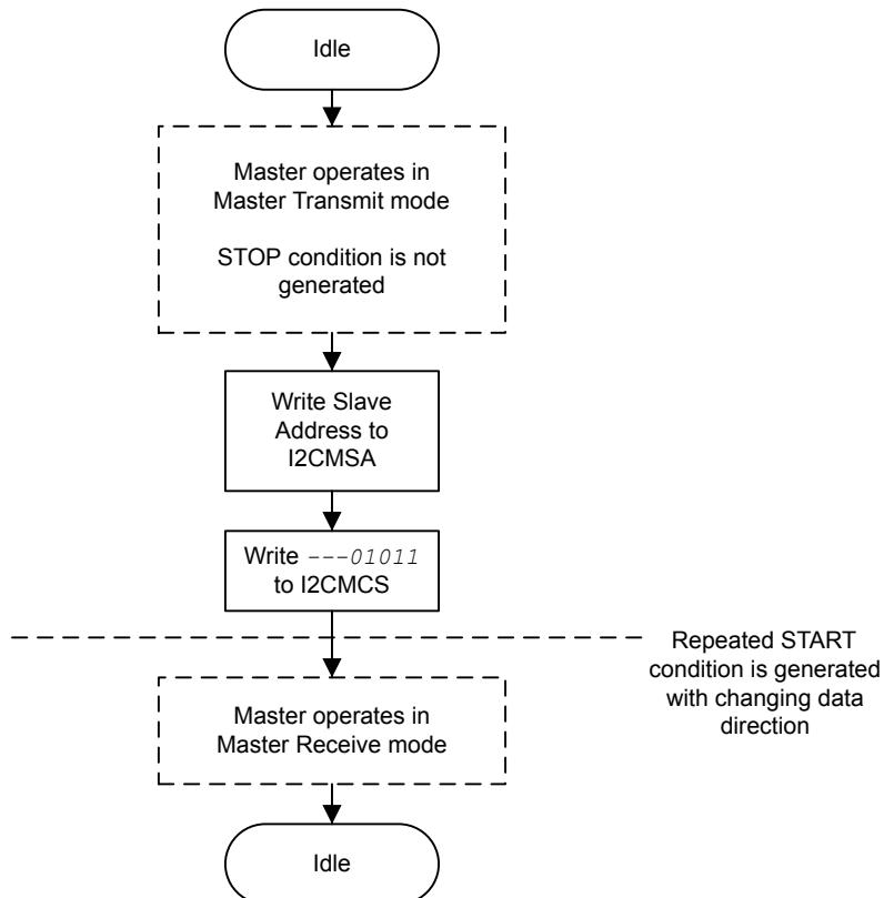
**Figure 21-13. Master TRANSMIT with Repeated START after Master RECEIVE**
