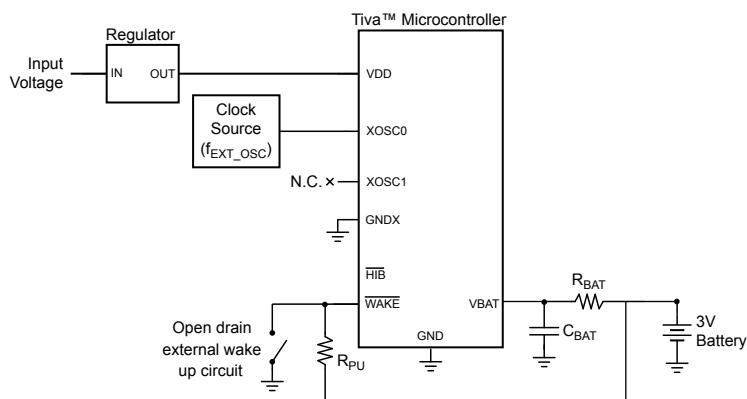
**Note:** Some devices may not supply a GNDX signal. See "Signal Tables" on page 1896 for pins specific to your device.
