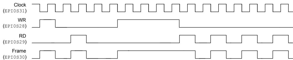
If the FRMCNT field is 0x1, then the FRAME signal pulses high during every other read or write access, see Figure 11-23 on page 860.
