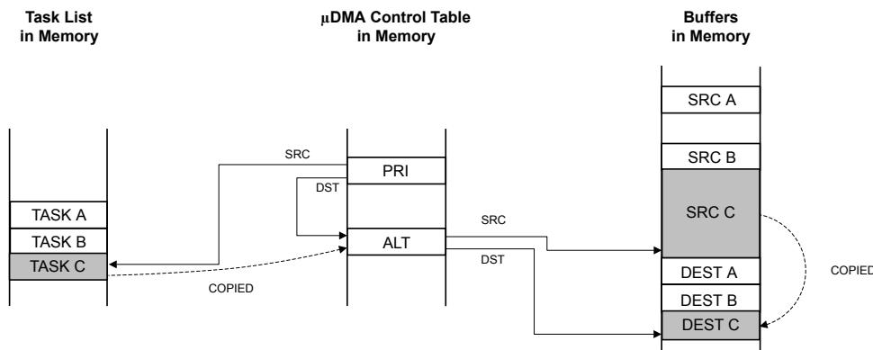
Using the channel's primary control structure, the μDMA controller copies task C configuration to the channel's alternate control structure.
