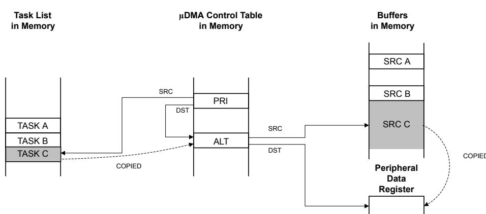
Using the channel's primary control structure, the  $\mu$ DMA controller copies task C configuration to the channel's alternate control structure.
