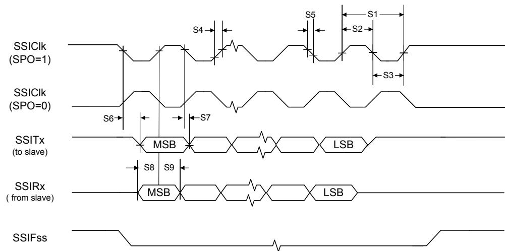
**Figure 30-32. Slave Mode SSI Timing for SPI Frame Format (FRF=00), with SPH=1**
