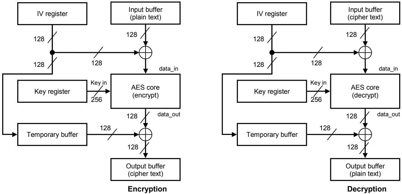
**Note:** The IV is created with an initial encryption, followed by an LFSR operation for each new block.
