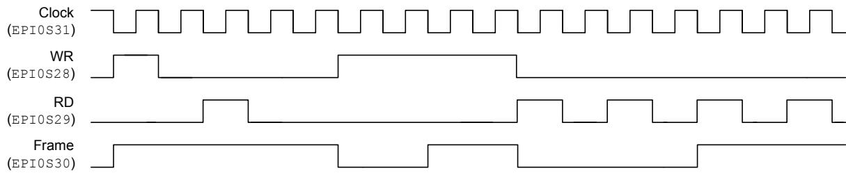
When **FRMCNT=2**, the FRAME signal transitions the rising edge of the WR or RD strobes for every third access, and so on for every value of **FRMCNT**, see Figure 11-27 on page 861.
