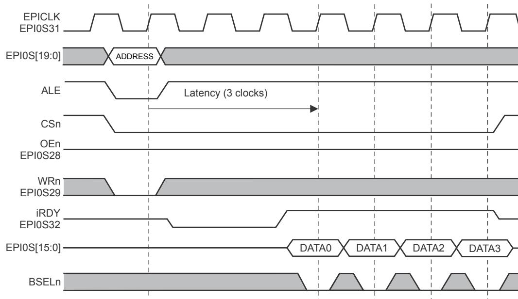
Note that if a read or write transfer attempts to begin during a refresh event, the transfer is held off by the assertion of the iRDY pin by the memory to the EPI module. Figure 11-9 on page 848 and Figure 11-10 on page 849 depict the delay in data transfer during a refresh collision.
