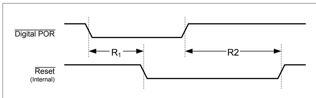
The digital Power-On Reset is only released when the analog Power-On Reset has deasserted and all of the Power-OK monitors for each of the supplies indicate that power levels are in operational ranges.
