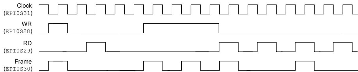
If the FRMCNT field is 0x2 and FRM50 is clear, then the FRAME signal pulses high during every third access, and so on for every value of FRMCNT, see Figure 11-24 on page 860.
