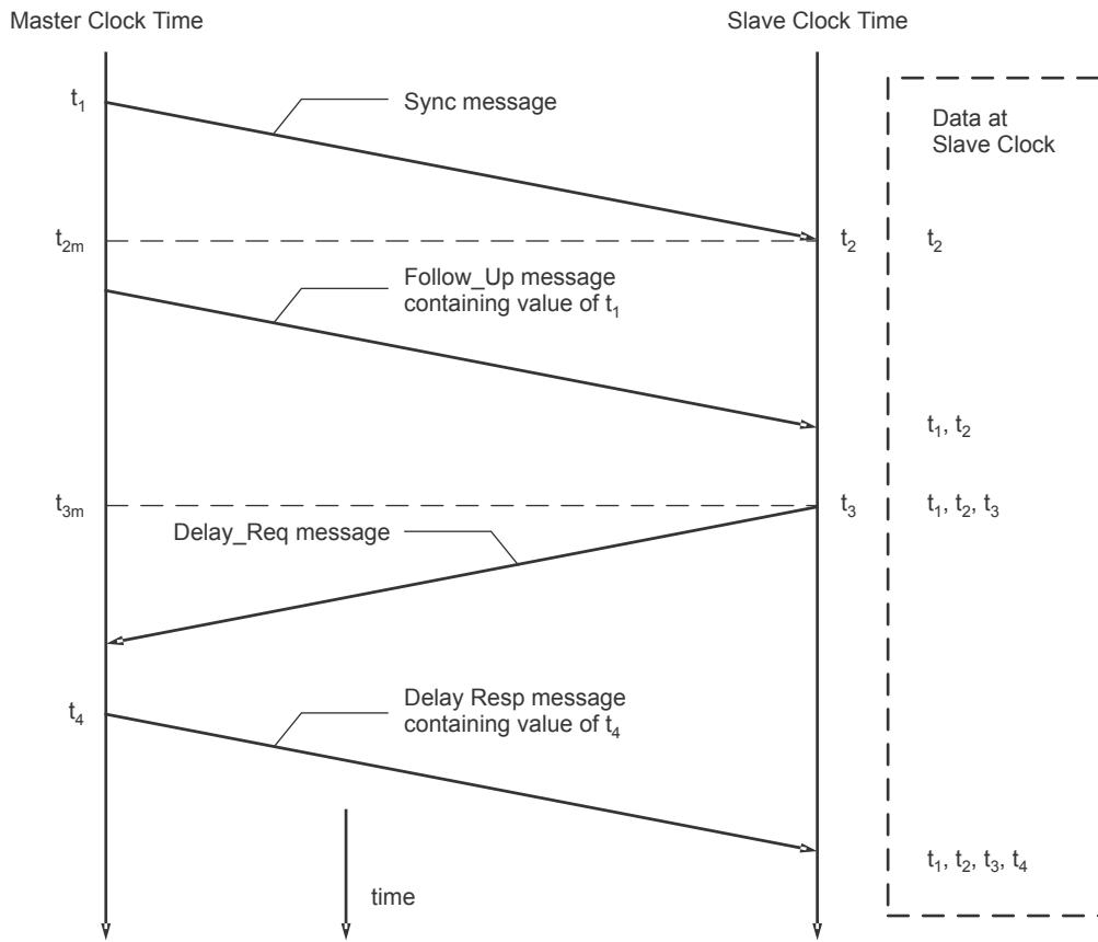
As shown in Figure 23-8 on page 1565, the PTP uses the following process:
