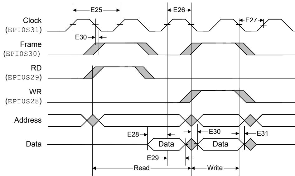
**Note:** This figure illustrates accesses where the FRM50 bit is clear, the FRMCNT field is 0x0 and the WR2CYC bit is clear.
