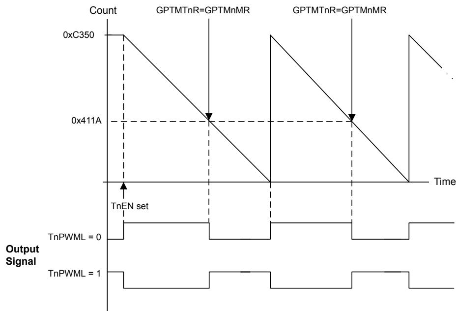
When synchronizing the timers using the **GPTMSYNC** register, the timer must be properly configured to avoid glitches on the CCP outputs. Both the **TnPLO** and the **TnMRSU** bits must be set in the **GPTMTnMR** register. Figure 16-5 on page 1091 shows how the CCP output operates when the **TnPLO** and **TnMRSU** bits are set and the **GPTMTnMATCHR** value is greater than the **GPTMTnILR** value.
