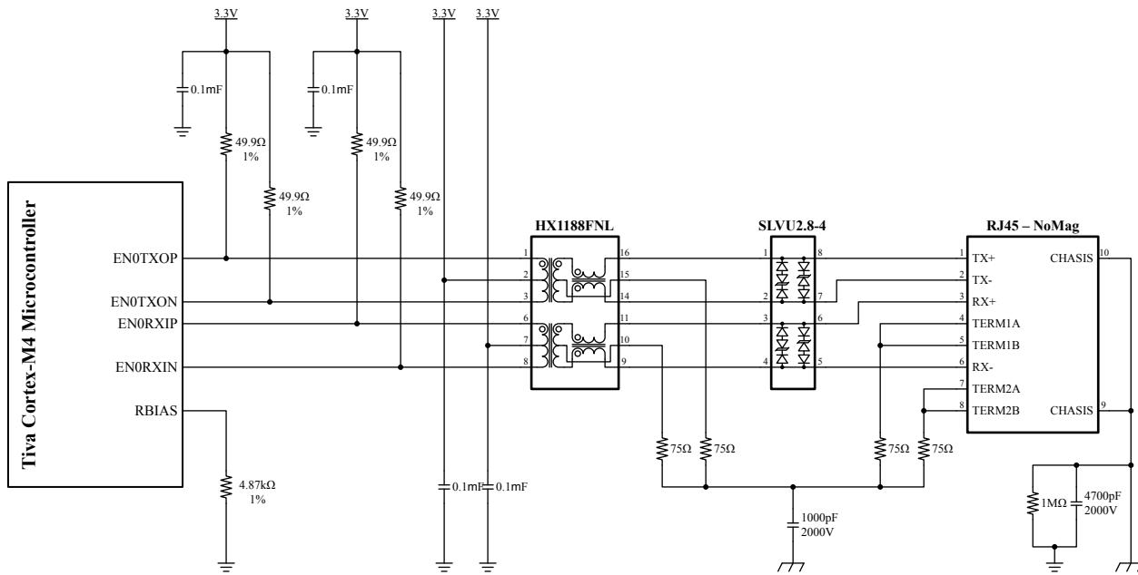
The Ethernet PHY is designed to work with transformers that meet the IEEE 802.3 standard. To utilize the Auto-MDIX (AMDIx) capability of the Ethernet PHY, a symmetrical transformer is recommended. The Pulse HX1188 transformer has been tested and is known to successfully interface to the Ethernet PHY.
