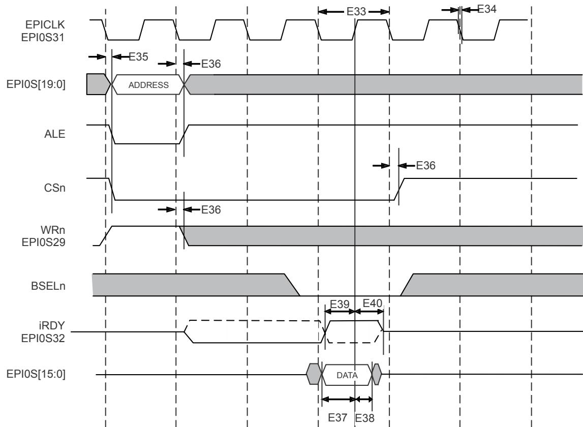
**Figure 30-27. PSRAM Single Burst Write**
