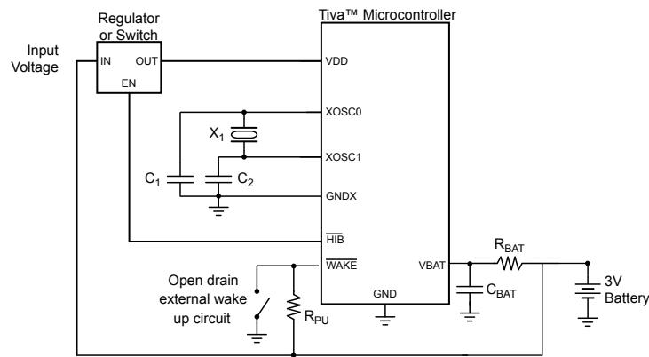
**Note:** Some devices may not supply the GNDX signal. If GNDX is absent, the crystal load capacitors can be tied to GND externally. See "Signal Tables" on page 1896 for pins specific to your device.
