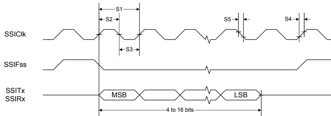
**Figure 30-31. Master Mode SSI Timing for SPI Frame Format (FRF=00), with SPH=1**
