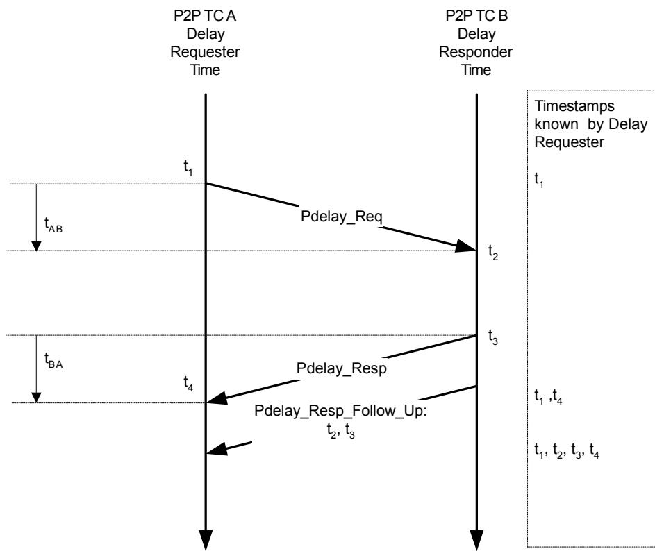
As shown in Figure 23-10 on page 1570, the propagation delay is calculated in the following way:
