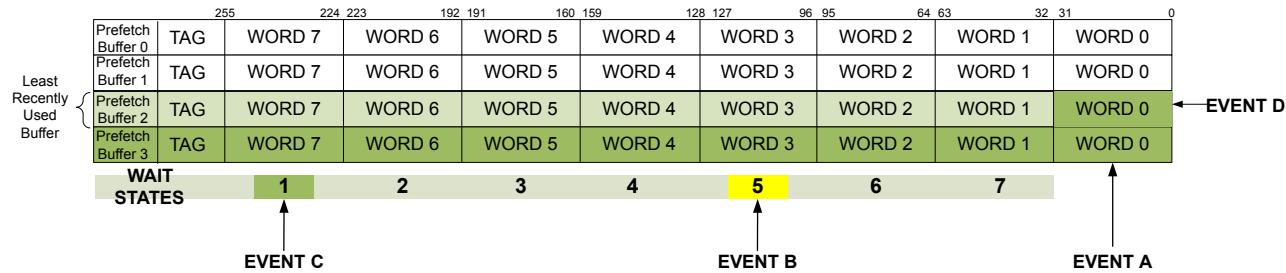
Note that if the CPU target word is beyond Word 2 (Word 3 through Word 7) then the next prefetch fill begins immediately and, depending on the CPU frequency, a delay is incurred between CPU access of Word 7 and Word 0 of the next line.
