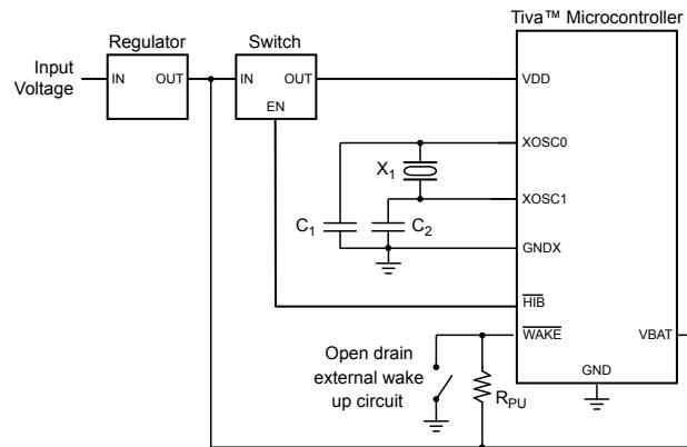
**Note:** Some devices may not supply a GNDX signal. See “Signal Tables” on page 1896 for pins specific to your device.
