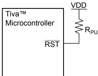
**Note:**  $R_{PU} = 0$  to  $100\text{ k}\Omega$
