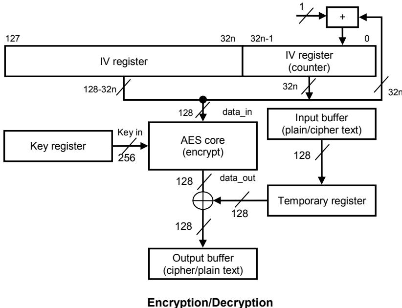
**Note:** The value for n can be 1, 2, 3, or 4 for CTR mode and is  $\frac{1}{2}$  for ICM mode.
