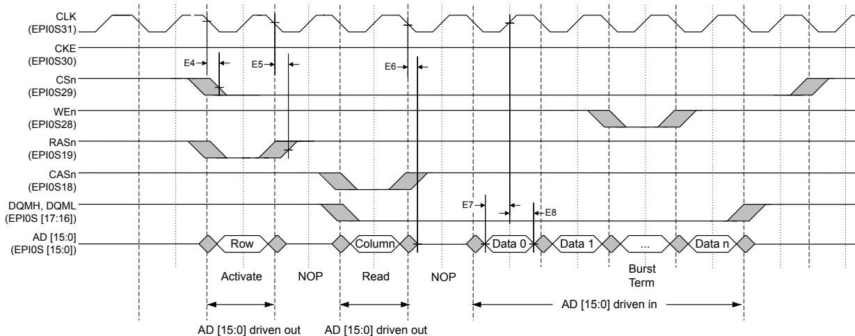
**Figure 30-20. SDRAM Write Timing**
