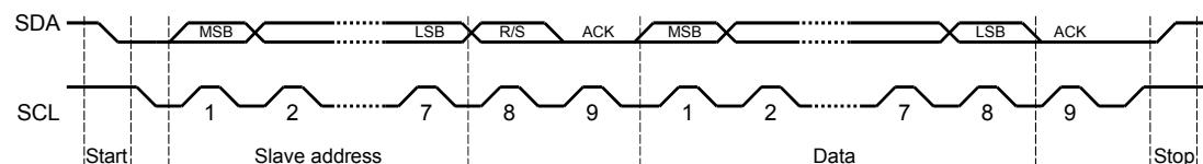
The first seven bits of the first byte make up the slave address (see Figure 21-5). The eighth bit determines the direction of the message. A zero in the R/S position of the first byte means that the
