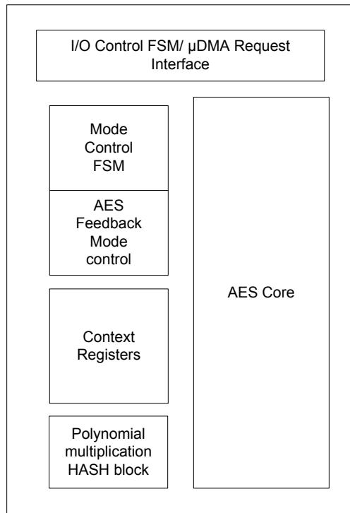
AES is an efficient implementation of the Rijndael cipher (the AES algorithm) and a 128-bit polynomial multiplication (referred to here as GHASH, as per the AES-GCM specification). Rijndael is a block cipher in which each data block is 128 bits. The polynomial multiplication multiplies two 128-bit vectors using the smallest 128-bit irreducible polynomial, represented by the following 128-bit string: {0<sup>120</sup>}||10000111. The two implementations are combined into the AES wide-bus engine.
