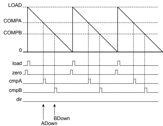
**Figure 26-4. PWM Count-Up/Down Mode**
