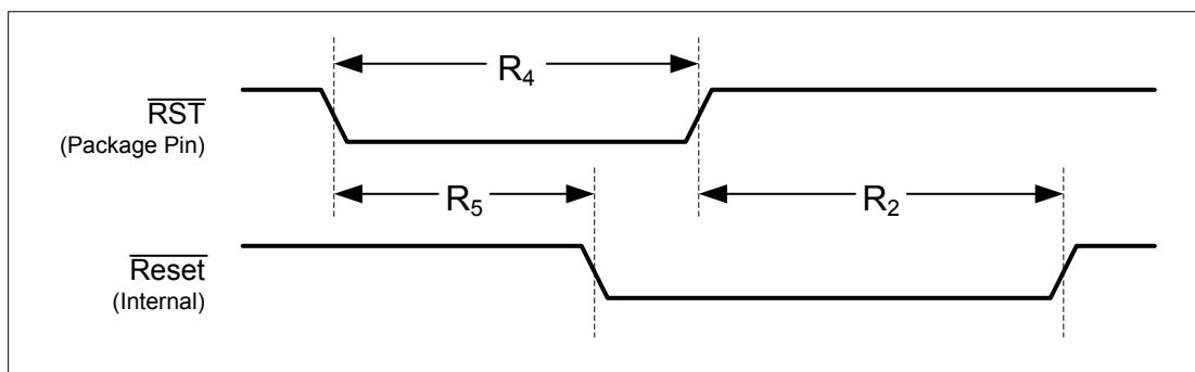
**Figure 30-12. Software Reset Timing**
