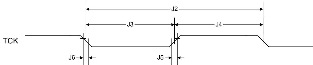
**Figure 30-3. JTAG Test Access Port (TAP) Timing**
