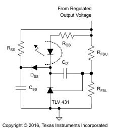
図 8-6. Example of Soft-Start Circuit Added to Error Amplifier
