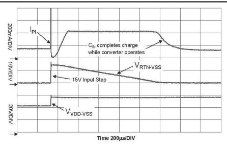
図 8-5. Response to PSE Step Voltage
