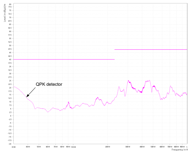
Figure 9-10. CISPR 32 Class B Radiated Emissions: Horizontal Polarization
