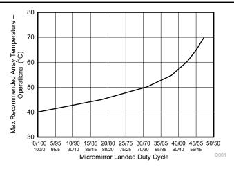
図 6-1. Maximum Recommended Array Temperature - Derating Curve
