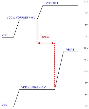
Refer to  ${\rm \clip{\sharp}}$  9-1 for  ${\rm V}_{\rm OFFSET}$  and  ${\rm V}_{\rm BIAS}$  supply voltage levels during power-up sequence delay.
