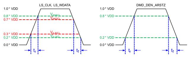
図 6-3. LPSDR Input Rise and Fall Slew Rate
