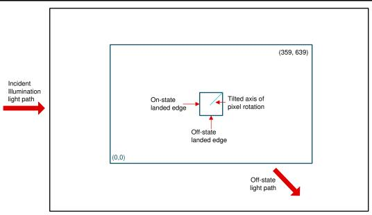
図 6-17. Landed Pixel Orientation and Tilt
