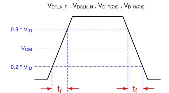
図 6-4. SubLVDS Input Rise and Fall Slew Rate
