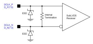
図 6-10. SubLVDS Equivalent Input Circuit
