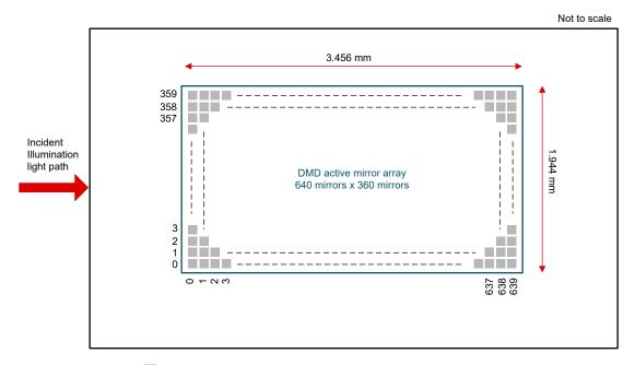
図 6-15. Micromirror Array Physical Characteristics
