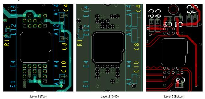
図 10-1. Power Supply Connections
