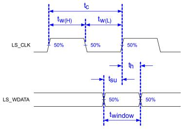
Low-speed interface is LPSDR and adheres to the セクション 6.6 and AC/DC Operating Conditions table in JEDEC Standard No. 209B, Low Power Double Data Rate (LPDDR) JESD209B.
