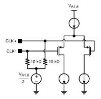
Figure 32. Equivalent Clock Receiver
