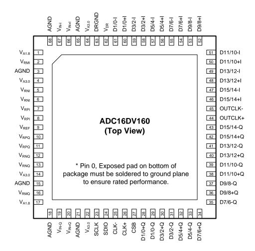
Figure 2. Pin-Out of ADC16DV160 See Package Number NKE0068A
