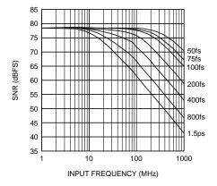
Figure 35. SNR with given Jitter vs. Input Frequency
