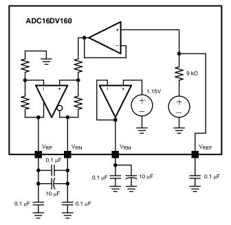
Figure 36. Internal References and their Decoupling
