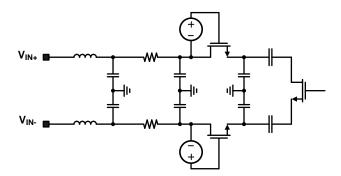
Figure 30. Input Equivalent Circuit
