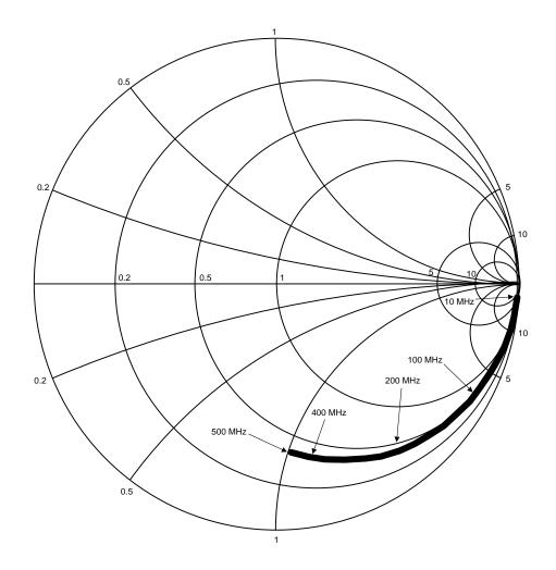
Figure 31. ADC16DV160 Input S11
