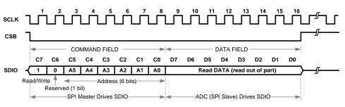
Figure 38. Serial Interface Protocol (Read Operation)
