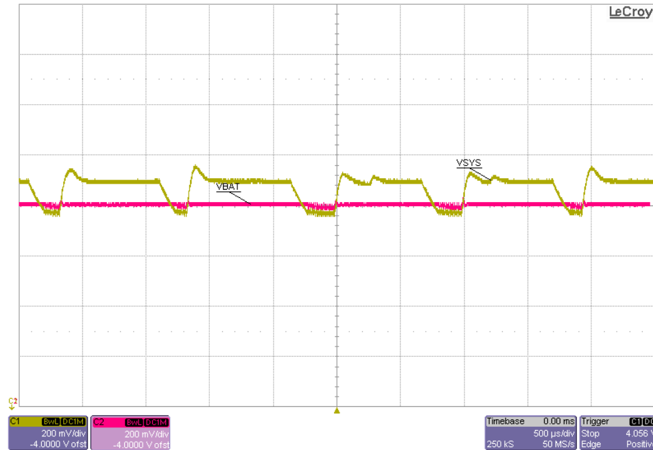
图 8-7. V(SYS) When Reverse Boost Prevention Circuit is Active
