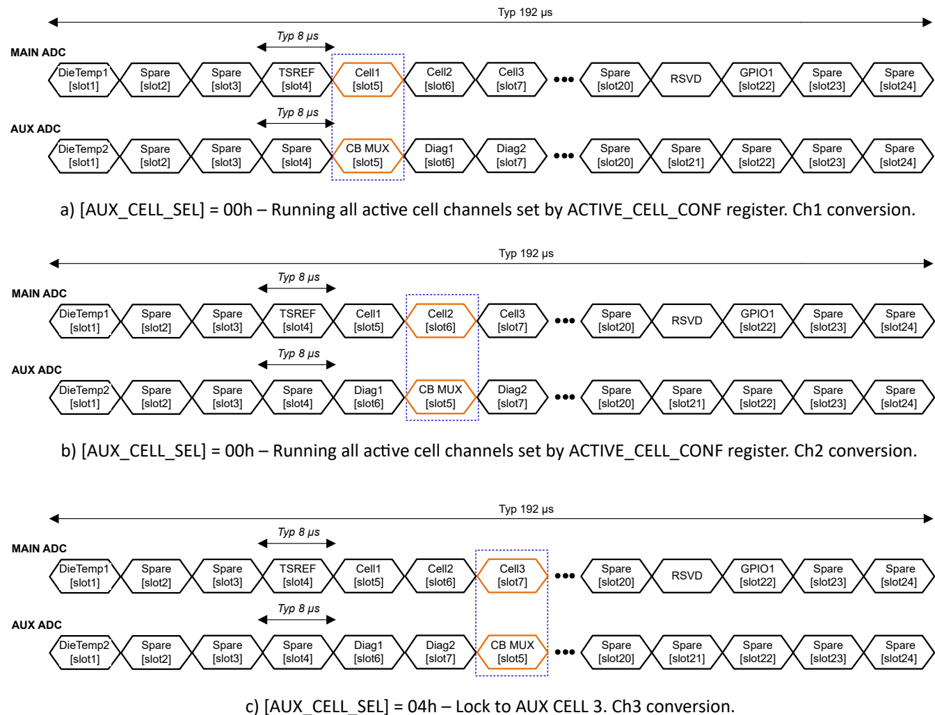
図 8-11. Synchronization Between MAIN and AUX ADC Sampling
