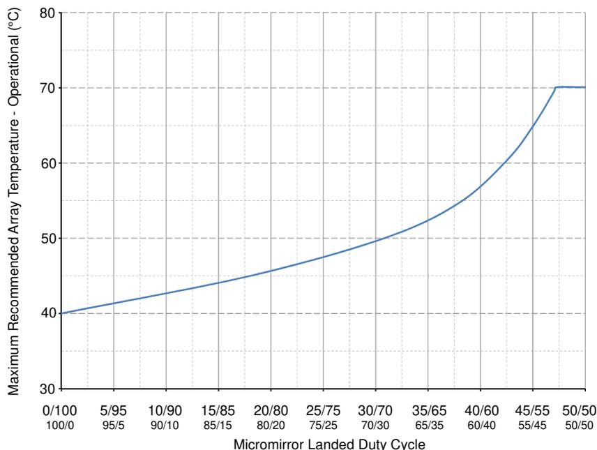
**5-1. Maximum Recommended Array Temperature—Derating Curve**
