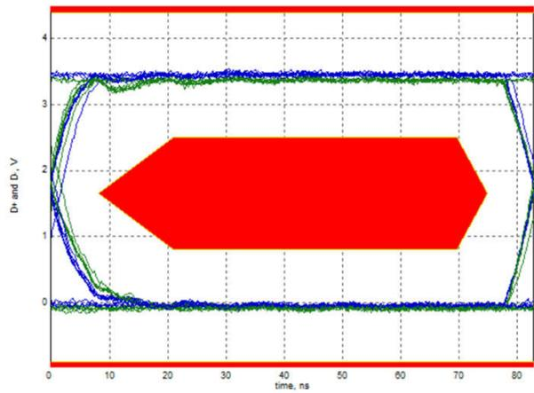
Figure 5-4. Typical Full-Speed (12 Mbps) Eye-Diagram through ISOUSB211-Q1
