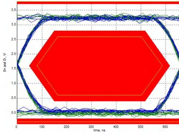
Figure 5-5. Typical Low-Speed (1.5 Mbps) Eye-Diagram through ISOUSB211-Q1
