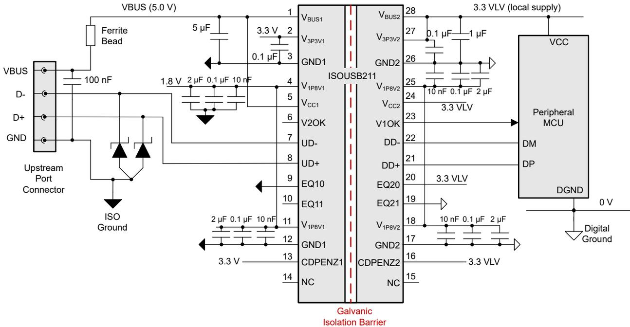
**Figure 8-6. Using ISOUSB211-Q1 without External 1.8-V Regulators**
