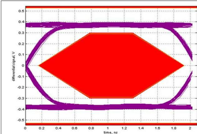
Figure 5-3. Typical High-Speed (480 Mbps) Eye-Diagram through ISOUSB211-Q1
