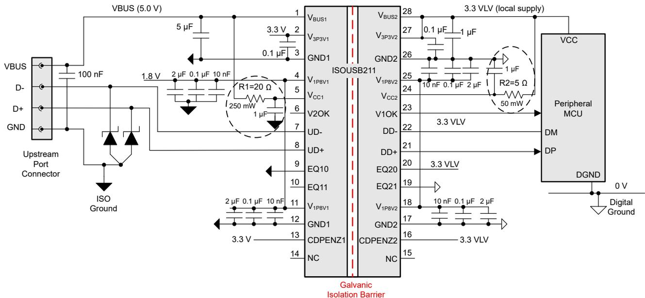
**Figure 8-8. Using ISOUSB211-Q1 with Resistors in series with V<sub>CCx</sub> pins**
