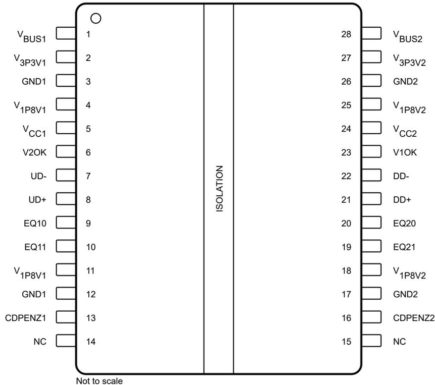
**Figure 4-1. DP Package 28-Pin SSOP Top View**
