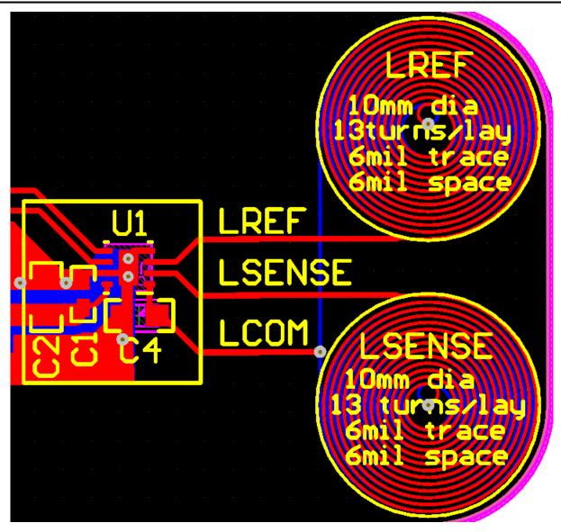
Figure 7-10. Side by Side Coil Layout Example
