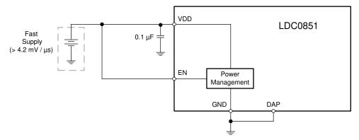
Figure 7-8. Supply Connections for Fast Ramp Rate
