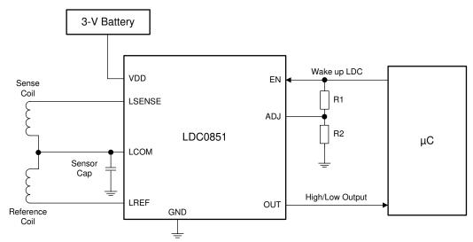
Figure 7-6. Application Schematic Showing Low Power Operation
