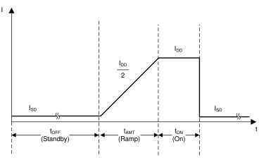
Figure 7-7. LDC0851 Supply Current vs. Time During Duty Cycle Operation
