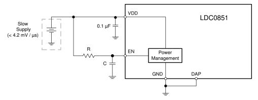
Figure 7-9. Supply Connections for Slow Ramp Rate
