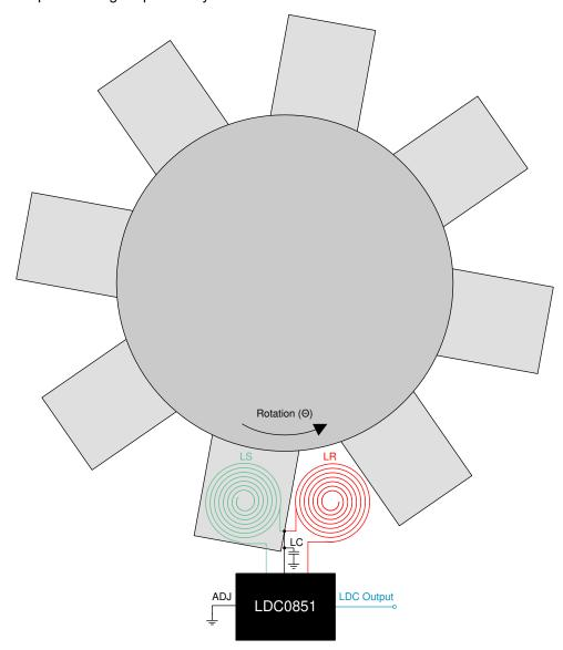
Figure 7-2. Gear Tooth Functional Diagram
