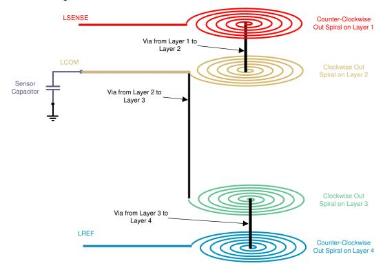
Figure 7-11. Stacked Coil Recommended Connections and Direction
