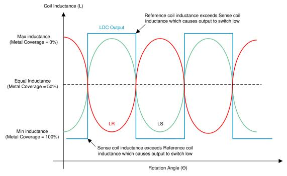
Figure 7-3. Angular Position vs Coil Inductance
