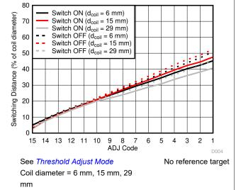
Figure 5-4. Normalized Switching Distance vs. ADJ Code
