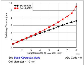
Figure 5-1. Switching Distance vs. LREF Target
