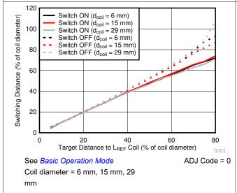
Figure 5-3. Normalized Switching Distance vs. LREF Target Distance
