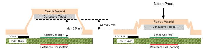
Figure 7-4. Coarse Position Sensing Side View
