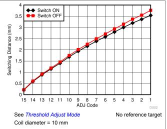
Figure 5-2. Switching Distance vs. ADJ code
