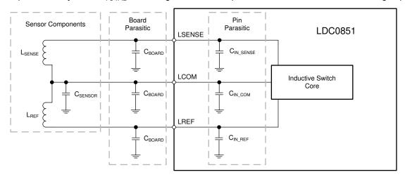
Figure 7-1. Sensor Components, Board Parasitics, and Package Parasitics Diagram
