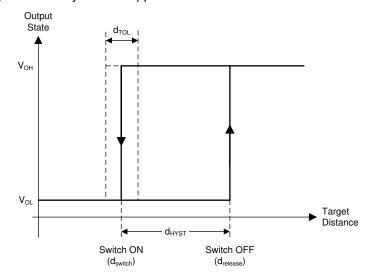
Figure 6-7. Switching Distance Hysteresis and Threshold Tolerance
